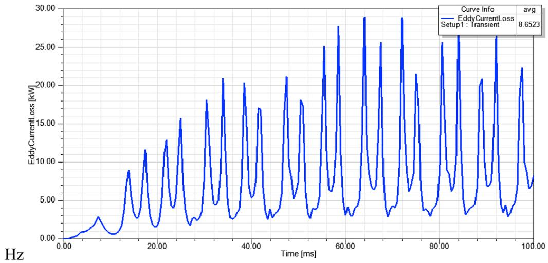
Fig. 7. Eddy loss of the model at a frequency of 50 Hz
