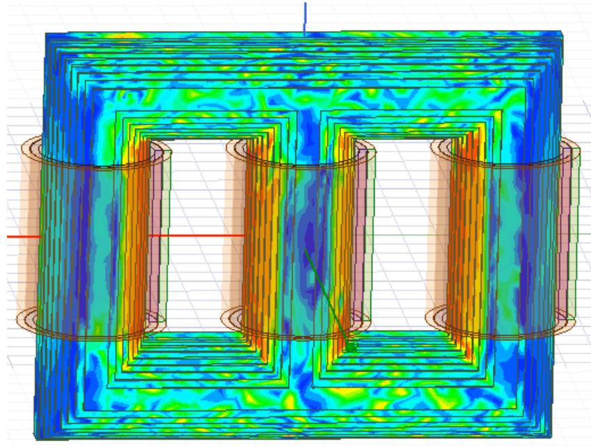
Fig. 13. Flux density distribution in 3D transformer model for 60 Hz frequency
