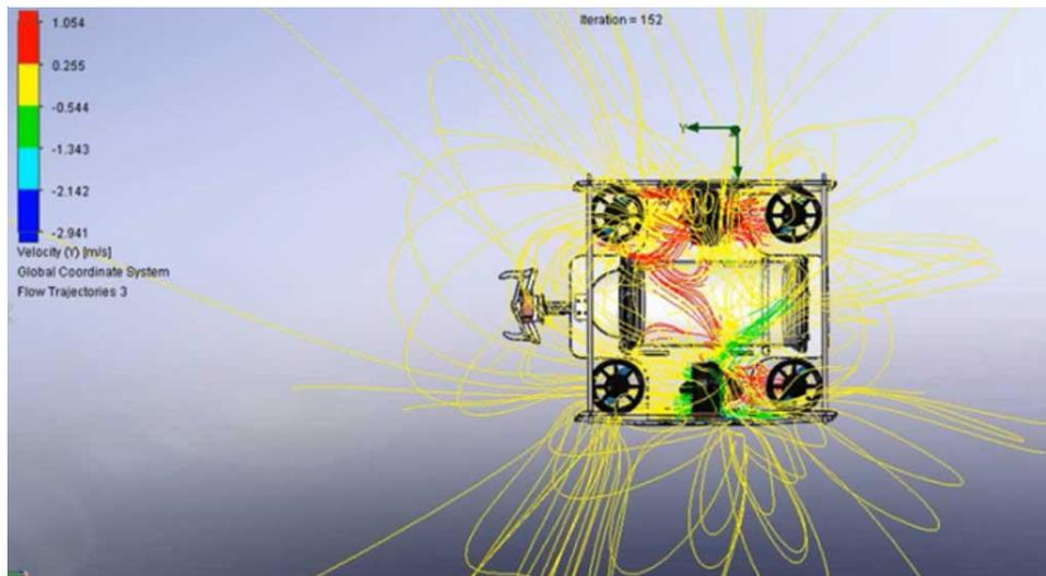
Figure 2. Visualization of flow lines formed during simulation
