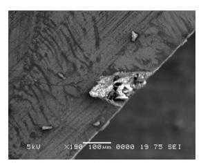
**Figure 1.** Notch wear initiation and propagation [6]
