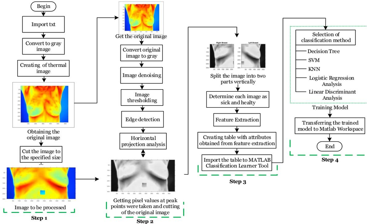
Figure 2. General working diagram of the developed system.
