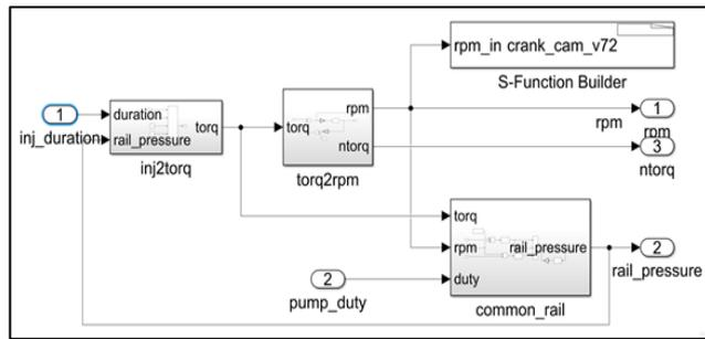
Figure 2. Engine model
