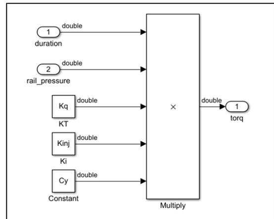
Figure 3. Injection duration to torque conversion
