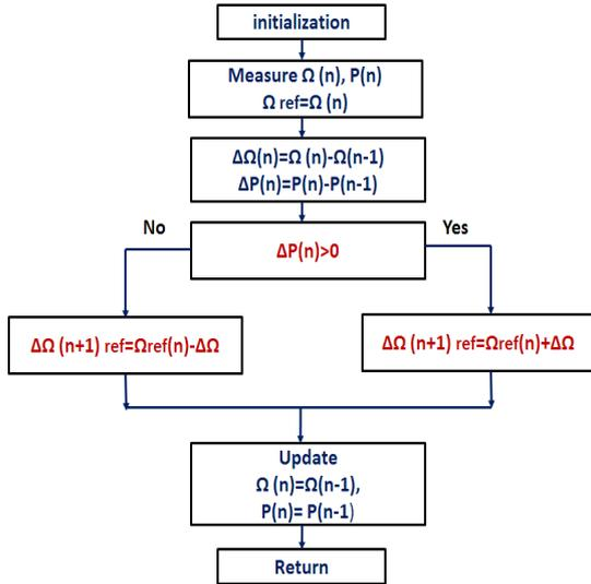
Figure 16. Flowchart of WECS algorithm.
