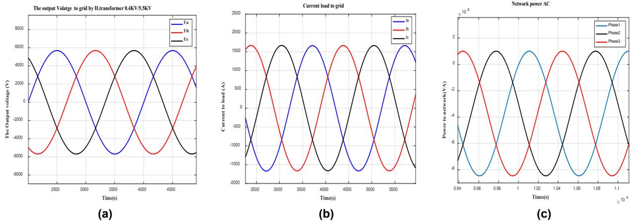
**Figure 32.** (a). Three-phase voltage of the distribution network. (b). Three-phase current of distribution network., (c). Three-phases Power AC network.
