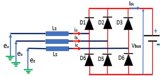
**Figure 6.** Diagram of a diode bridge three phases uncontrolled.
