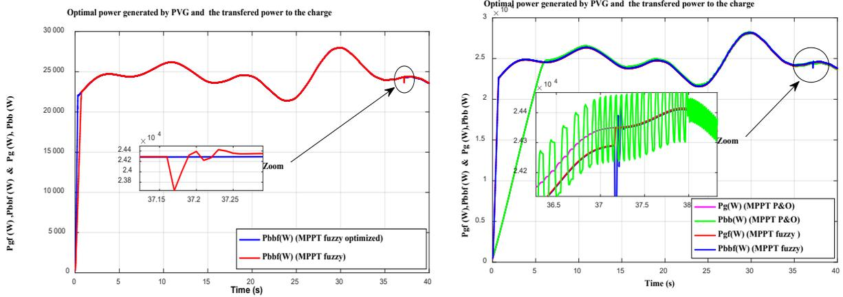
Figure 20. (a) . Power generated by PVG and the transferred power to the charge. (b) : Variations of the optimal power of PVG.
