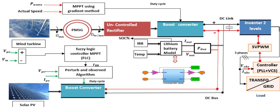
Figure 1. Hybrid power source (HPS) system.
