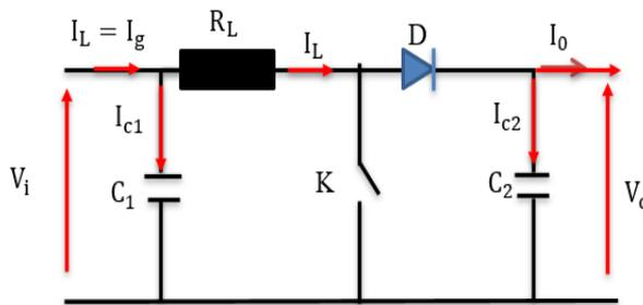
**Figure 9.** Electrical circuit of a boost converter.
