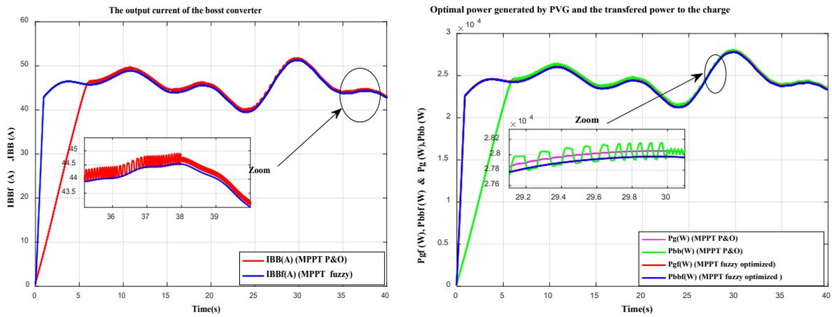
Figure 21. (a) . Charging current and voltage of battery. (b). Power of PVG transferred to the batteries issued by the FLC and FLC optimized
