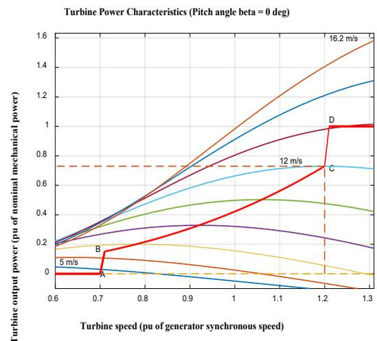
**Figure 15.** Turbine output power characteristics for the pitch angle  $\beta$ .
