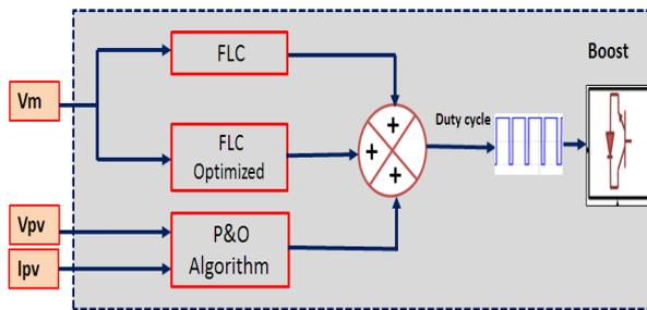
Figure 11. Block diagram of proposed MPPT approach for PV subsystem.
