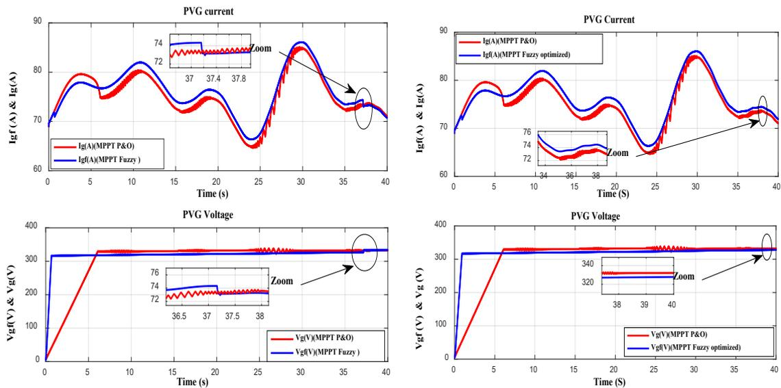
Figure 22. (a). Voltage & current of PVG with FLC. (b). Voltage & current of PVG with FLC optimized.
