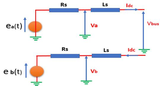
**Figure 7.** Equivalent diagram of a sequence in normal conduction.
