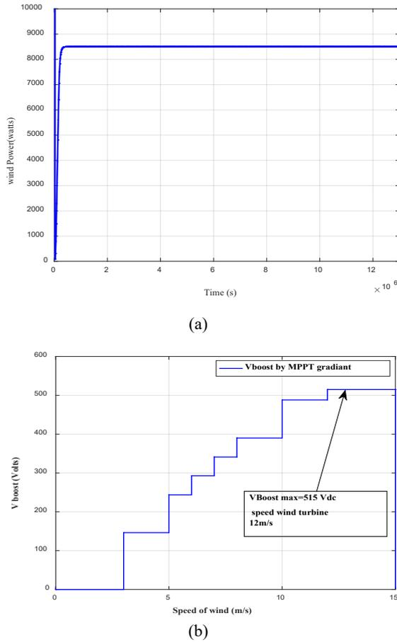
**Figure 8.** (a): Power of the wind turbine depending on the wind speed, (b): Variation of voltage Boost by speed wind turbine.
