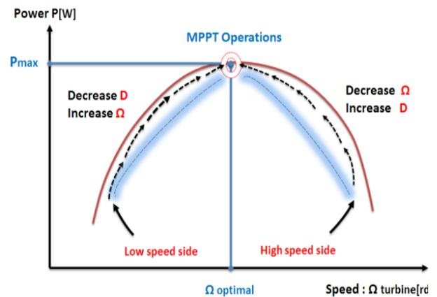
**Figure 14.** Wind power curve for an arbitrary wind speed.
