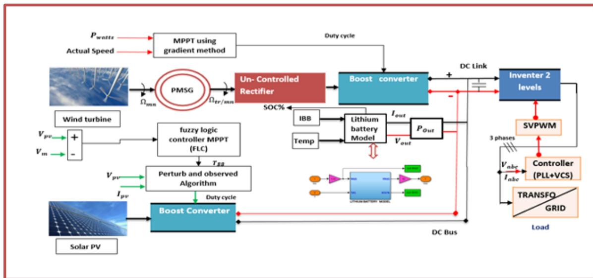
**Figure.** Schematic diagram of Proposed Hybrid System
