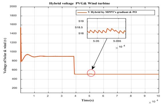
**Figure 26.** Variation of boost output voltage.
