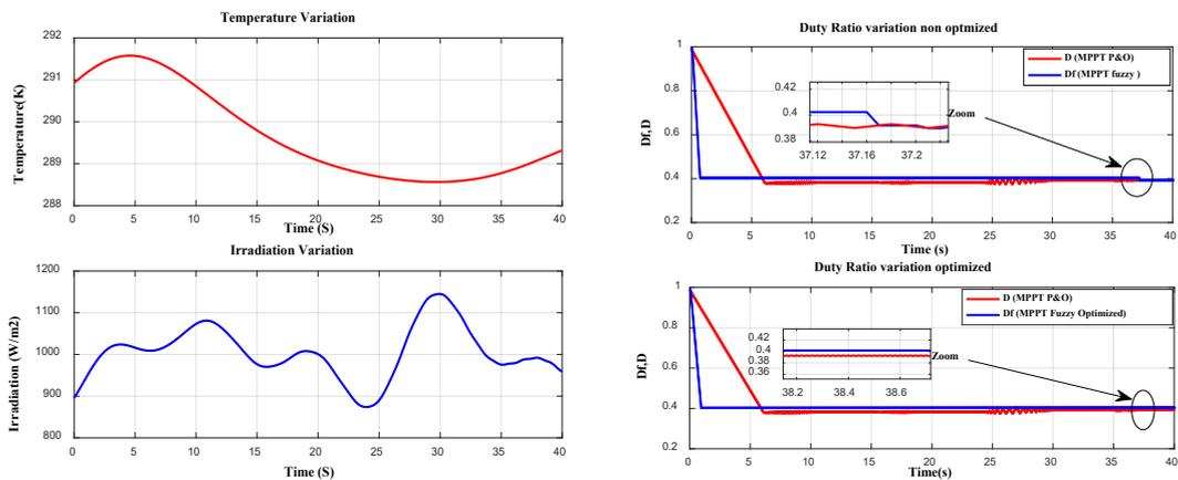
Figure 19. (a) . Variation of irradiation and temperature. (b). Duty Ratio Variation optimized.
