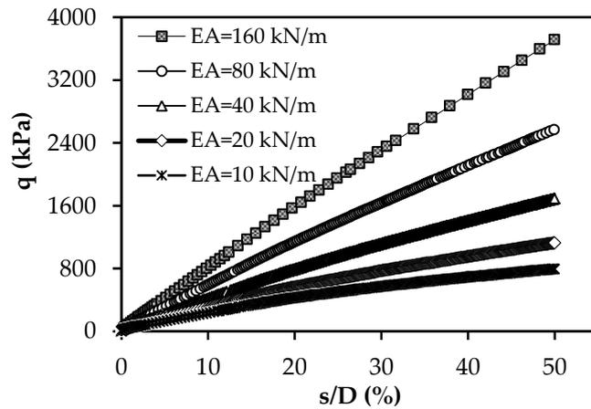
Figure 9. Geogrid stiffness effect on the column encasement
