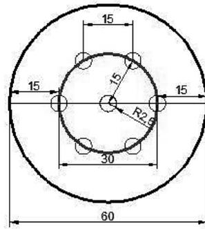
Figure 14. Arrangement of seven columns in a group
