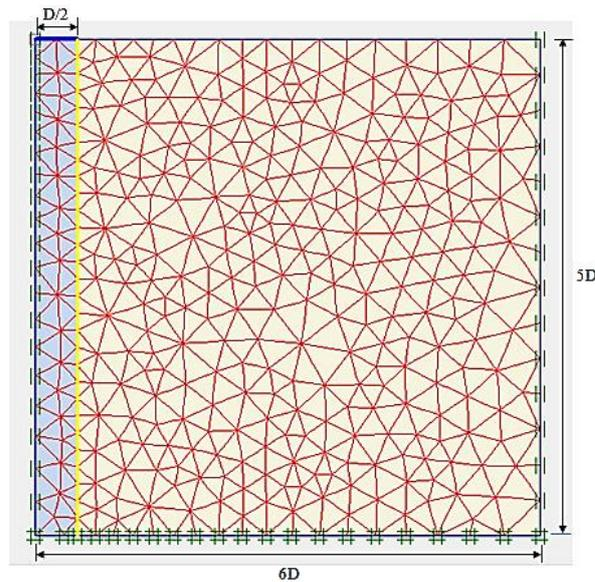
Figure 4. Finite element model in Plaxis
