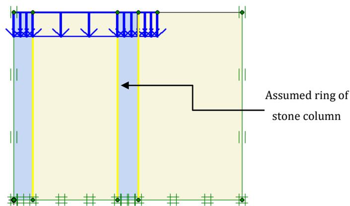
Figure 15. Finite element model in Plaxis for group column
