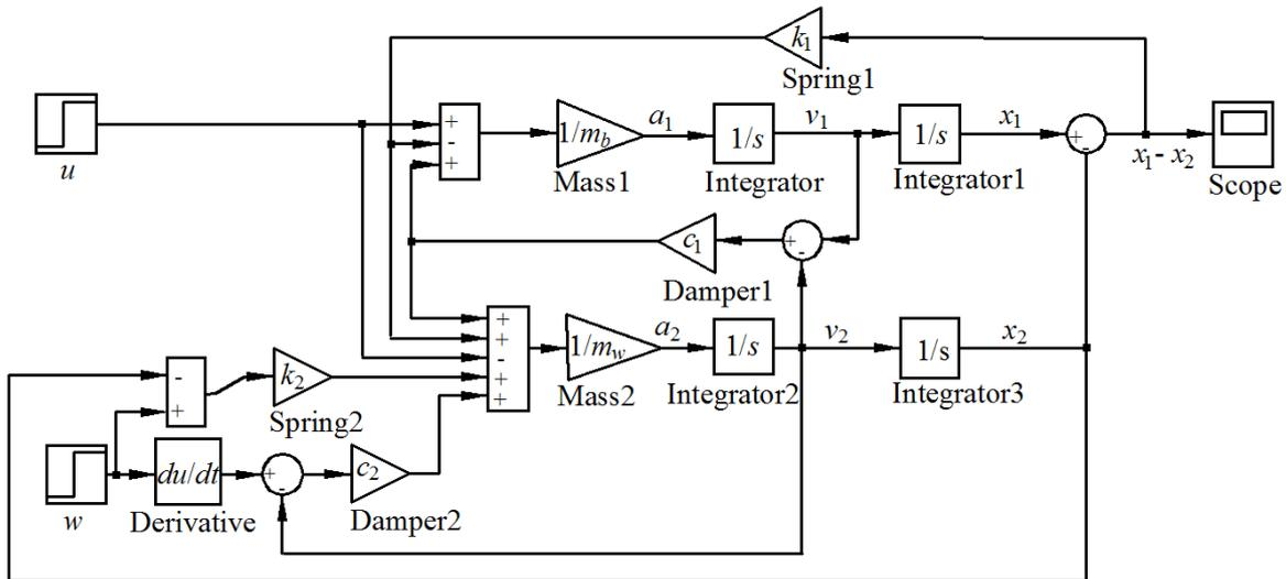
Fig. 4. Simulink model belonging to car suspension system
