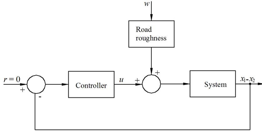
Fig. 2. Car suspension systems belonging to block diagram
