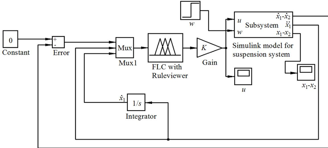
Fig. 7. The block diagram of the FLC model
