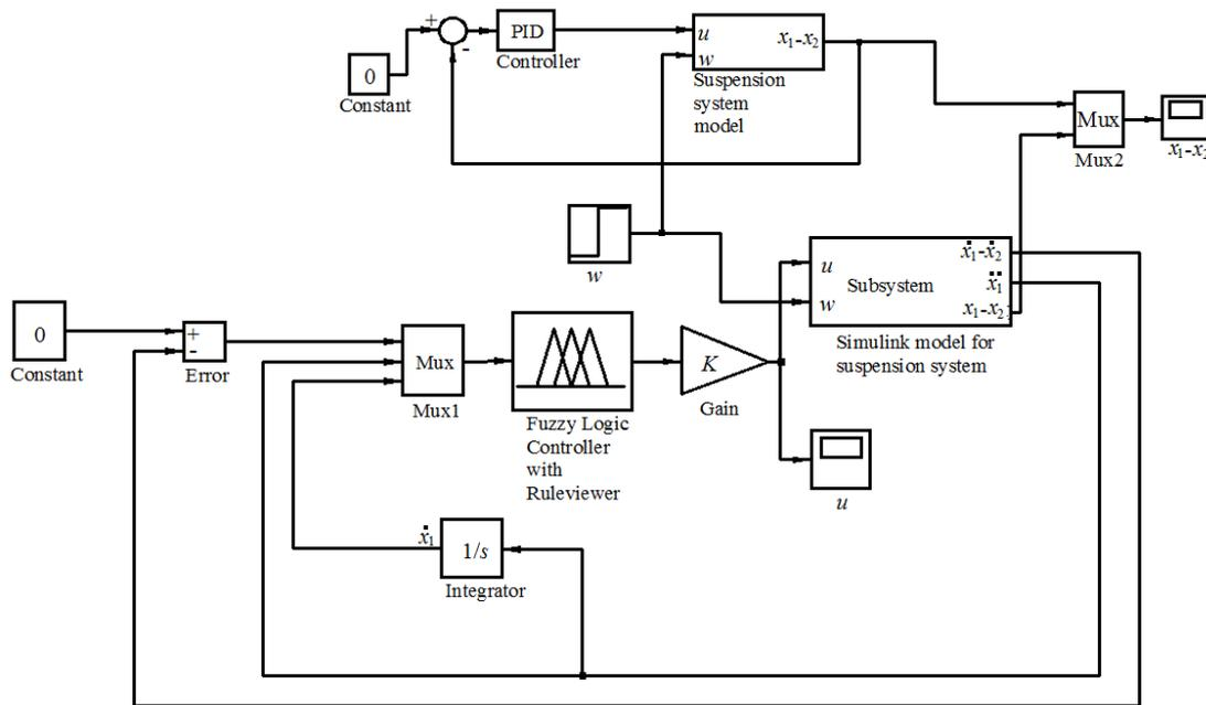
Fig. 9. Simulink model for PID and FLC controllers
