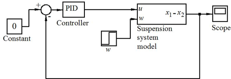
Fig. 3. PID controller Simulink model for suspension system
