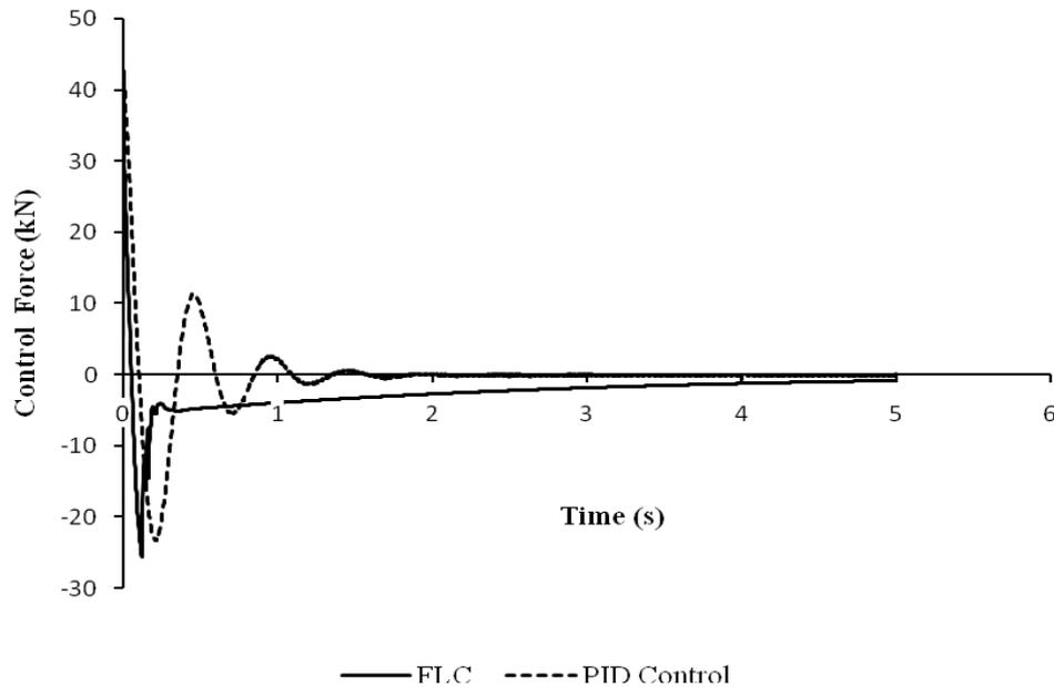
Fig. 11. Comparison of the control forces of PID and FLC controllers
