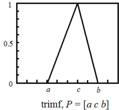
Fig. 6. Triangular type membership function and its parameters
