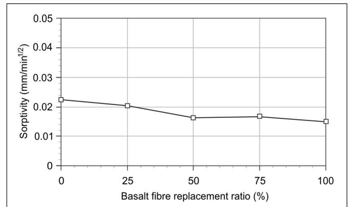
**Figure 6.** The variation of sorptivity values in terms of the basalt fibre replacement ratios.
