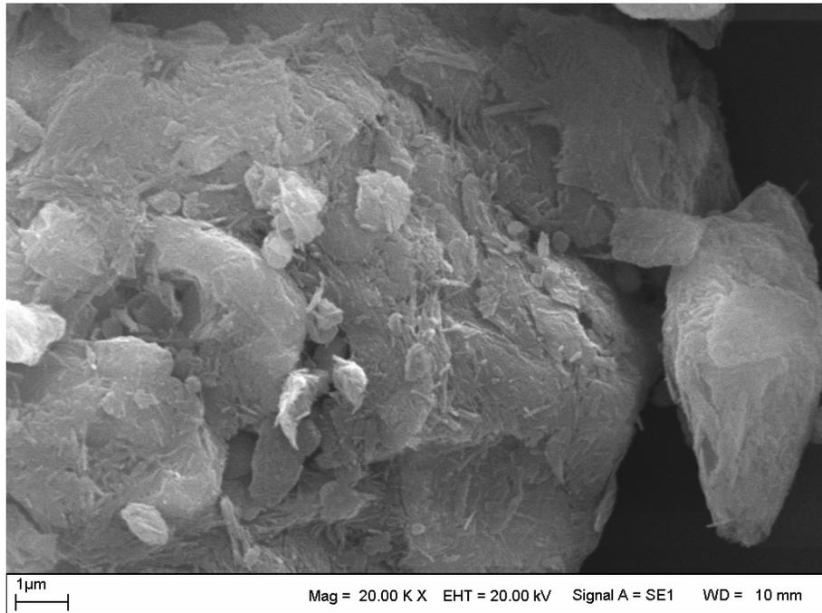
**Figure 1.** Scanning electron microscope image for red clay.
