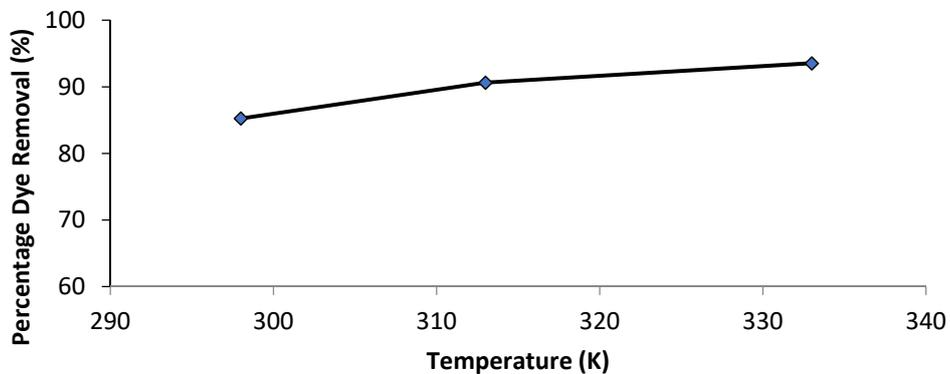
Figure 6. Effect of temperature ( $m = 1$  g,  $t = 1$  h, 400 rpm,  $C_0 = 100$  ppm).
