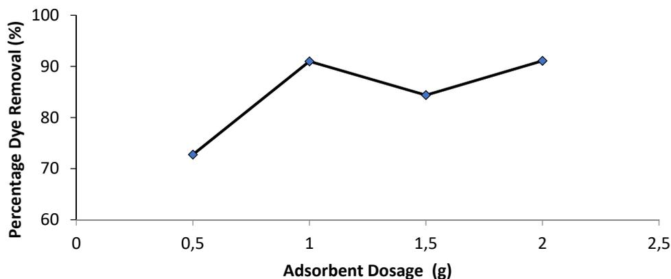
**Figure 4.** Effect of adsorbent dosage ( $t = 1$  h,  $T = 298$  K, 400 rpm,  $C_0 = 100$  ppm)
