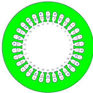
Figure 3. Stator and coil structure of motors.
