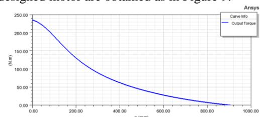
Figure 9. Torque-speed curves of the designed motor.
