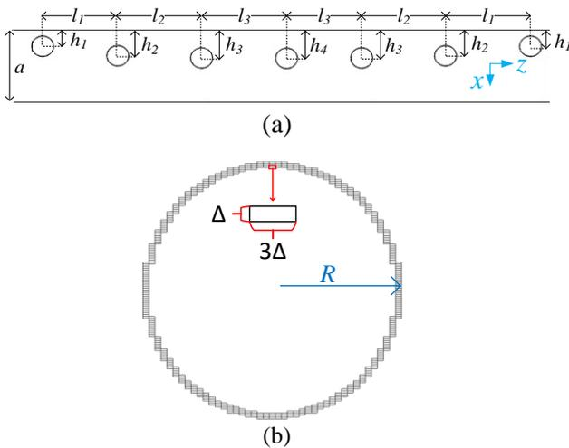
Figure 3 (a) Geometry of the metallic post filter with  $a = 22.86 \text{ mm}$ ,  $r = 3.21 \text{ mm}$ ,  $h_1 = 5.215 \text{ mm}$ ,  $h_2 = 8.172 \text{ mm}$ ,  $h_3 = 8.863 \text{ mm}$ ,  $h_4 = 8.971 \text{ mm}$ ,  $l_1 = 21.895 \text{ mm}$ ,  $l_2 = 24.461 \text{ mm}$ ,  $l_4 = 24.797 \text{ mm}$ , (b) mesh distribution of an equal cylinder in the system
