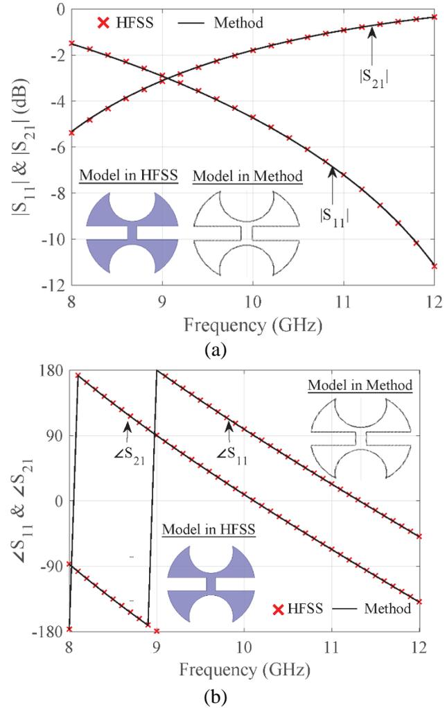
Figure 6 Comparison between the proposed method and HFSS for the frequency response of the arbitrarily shaped PEC object (a) magnitude (b) phase
