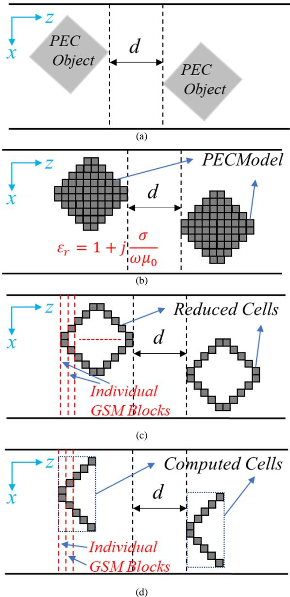
Figure 2 Example problem (a) original case (b) discretized PEC model (c) proposed approach with reduced cells (d) final computation case
