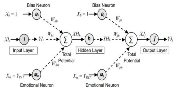
Figure 3 Process for EmNN feed-forward calculation [21-22]
