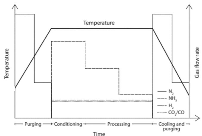
**Figure 2.** FNC process diagram of brake disc
