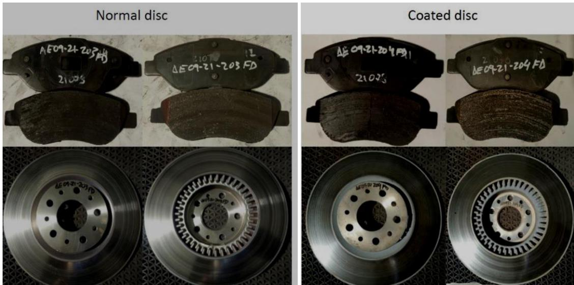
Figure 8. Disc-pad friction surfaces after wear test
