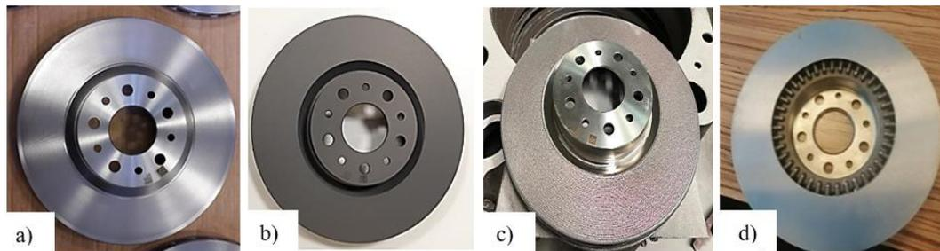
Figure 5. Brake disc surfaces a) uncoated b) FNC treated c) laser clad d) cladded after grinding
