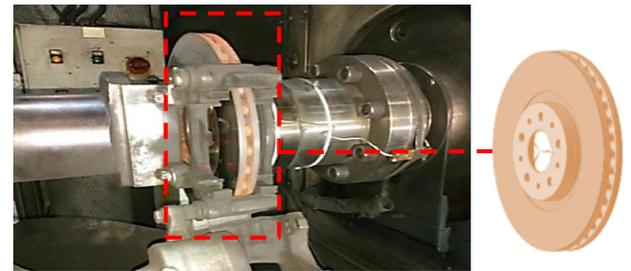
Figure 3. The brake disc on the brake performance test rig
