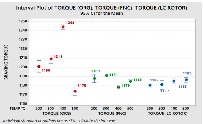
Figure 10. Brake torque variations at the elevated test temperatures
