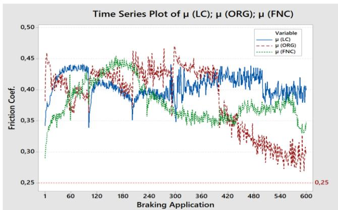
Figure 9. Disc-pad friction coefficient trend at the different braking cycles.
