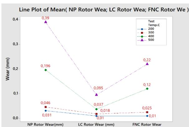
Figure 6. Wear comparison graph of rotors for uncoated disc-pad (NP) and coated disc-pad (LC) pairs at different temperatures.
