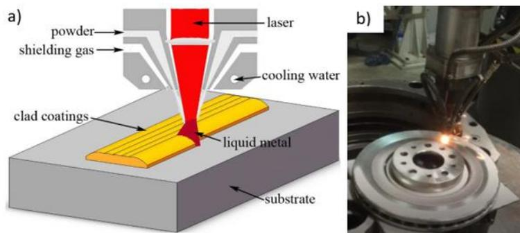
**Figure 1.** a) The schematic diagram of laser cladding [21] b) Brake disc laser cladding process.
