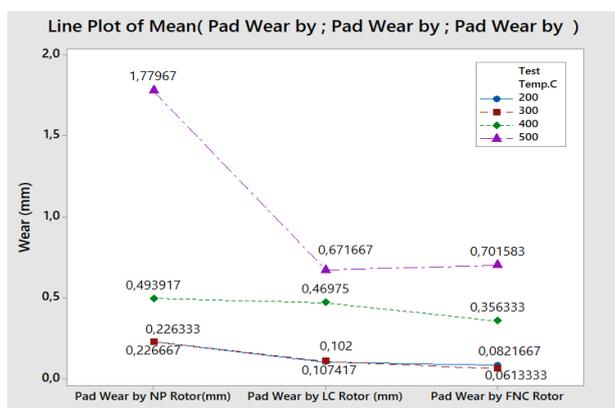
Figure 7. Wear comparison graph of pads for uncoated disc-pad (NP), coated disc-pad (LC) pairs, and coated disc-pad (FNC) pairs at different temperatures.
