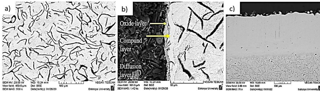
Figure 4. SEM analysis with a) laminar graphite cast iron b) coating layer treated by FNC c) laser clad layer.
