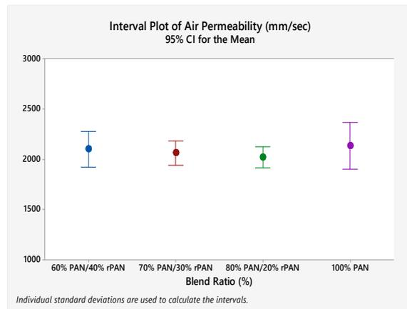
**Figure 6.** Air permeability results of yarn samples
