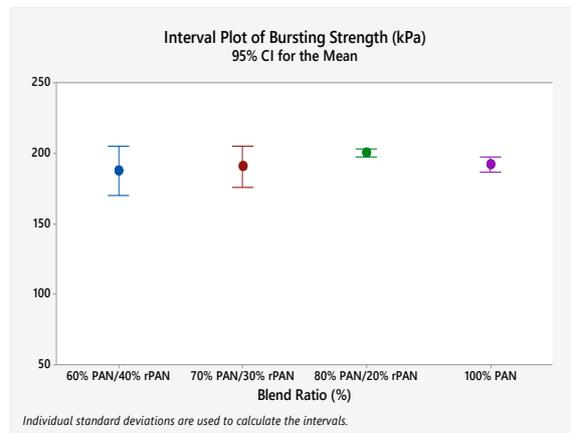
**Figure 7.** Bursting strength results of yarn samples
