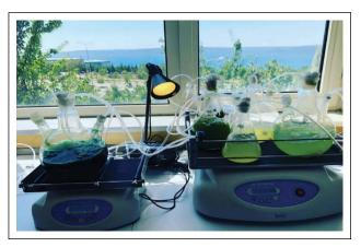
Figure 1. Microalgae adhesion test of the composite coating.
