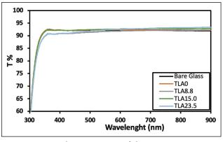
**Figure 2**. Optical transmission of the TEOS-LA composite films.
