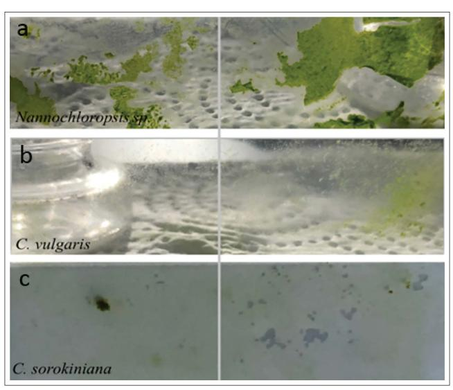
**Figure 4**. The biofouling performance of TLA<sub>18.7</sub> interaction with microalgae species. The left side is coated, and the right side is uncoated on images a) *Nannochloropsis sp.* b) *C. vulgaris*, and c) *C. sorokiniana*, respectively.
