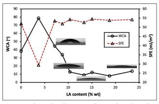
**Figure 3**. Changed with WCA and SFE values depending on the LA content of the composite films.
