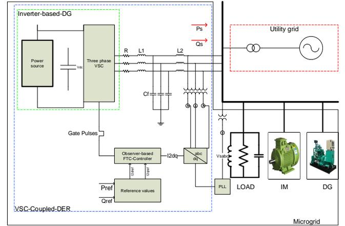
Fig. 1. The simulated grid-tied microgrid.
