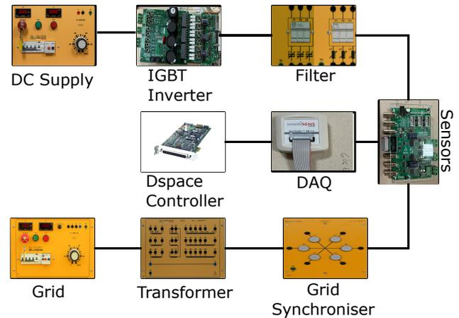
Fig. 6. Experimental Setup.
