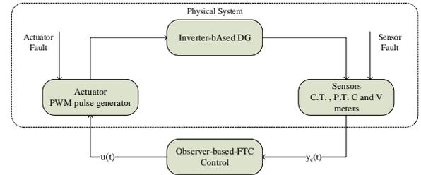
Fig. 2. FTC diagram of the VSC-coupled DER.
