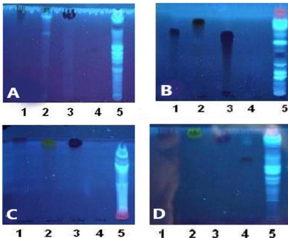
Based on these findings, we selected the combination of ethyl acetate, methanol, and distilled water (100:13.5:10) as it provided the best separation of the total polyphenolic extract of *H. tuberculatum* and the standard molecules used.
