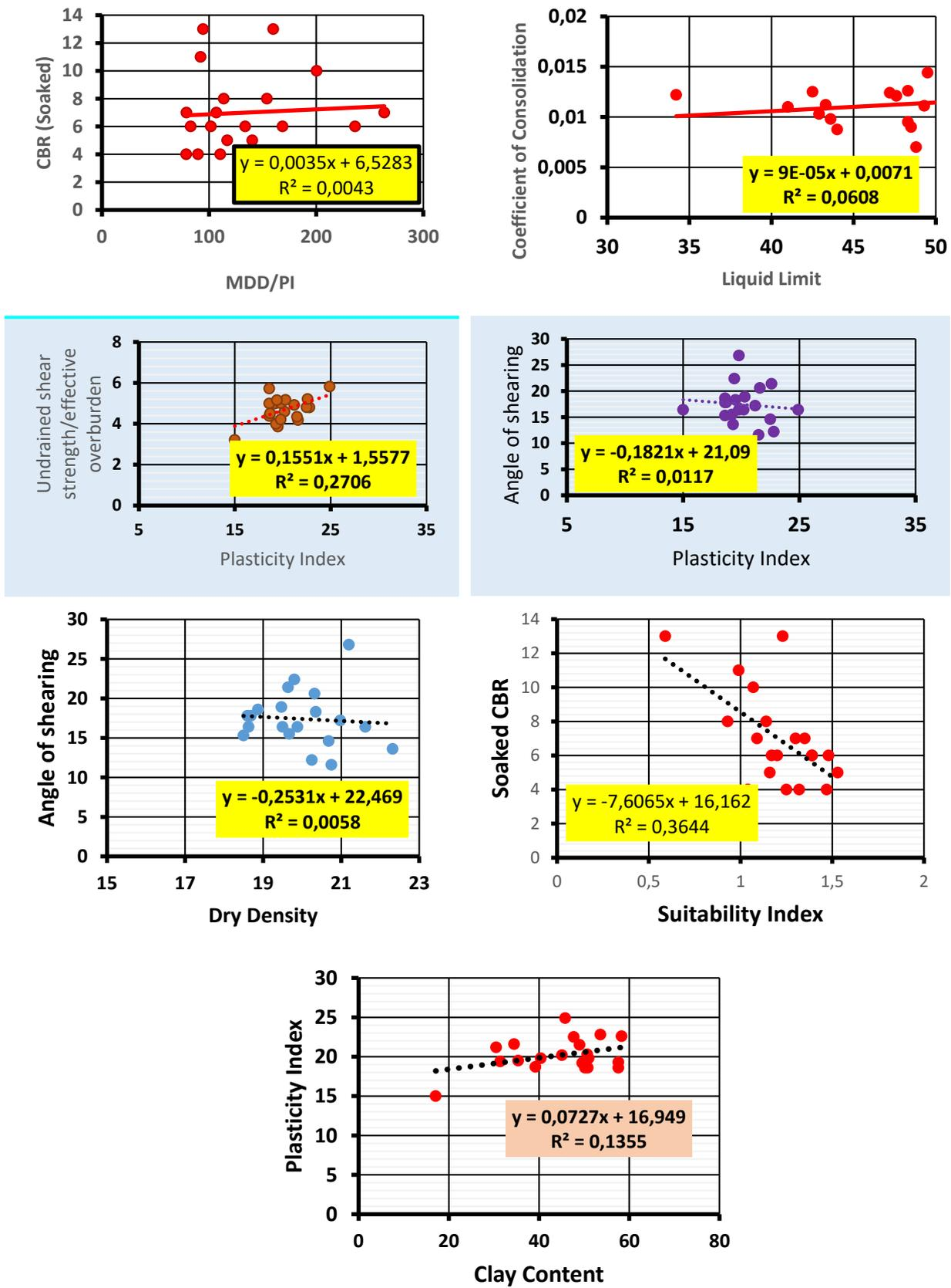
Fig. 10. Geotechnical parameters correlation for some of the engineering properties of the soils
