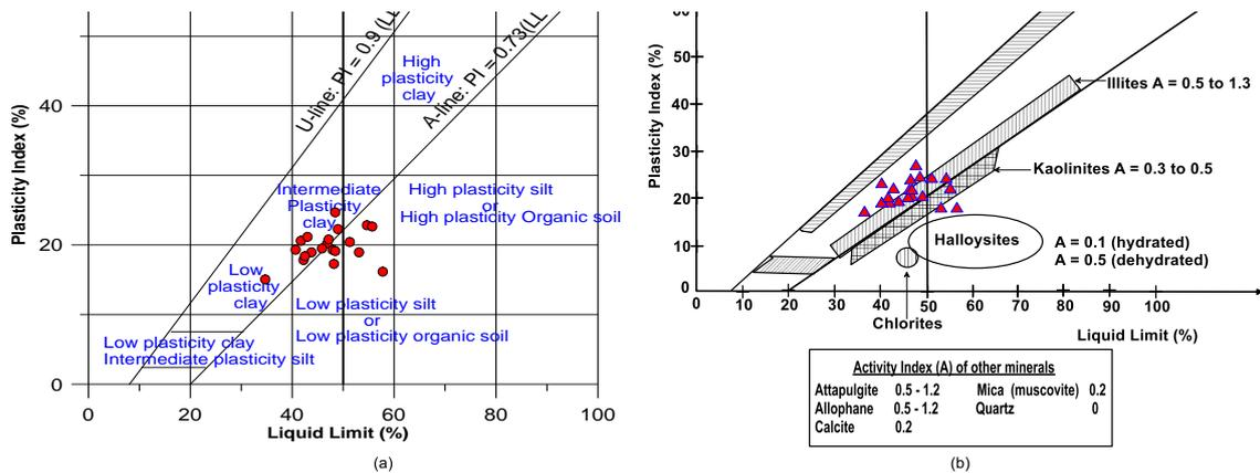
Fig. 8. (a) Plasticity Chart for the soil samples, showing prominent CL and CI plasticity group (b) Clay mineralogy group of the soil samples with most within Illite group
