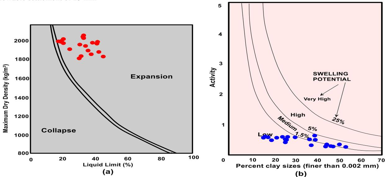
Fig. 12. Workability and swelling potential of the soils Classification chart for swelling potential (After Carter and Bentley, 1991; Holtz and Kovacs, 1981)
