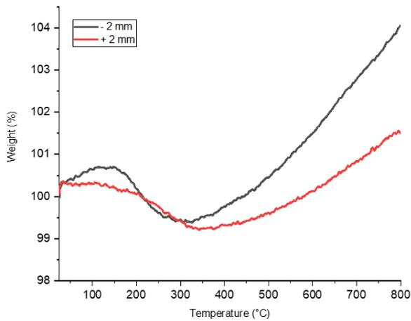
Figure 2. Thermo-gravimetric analysis -2 and +2 mm AlSi7Mg0.3 machining waste under pure O<sub>2</sub>.
