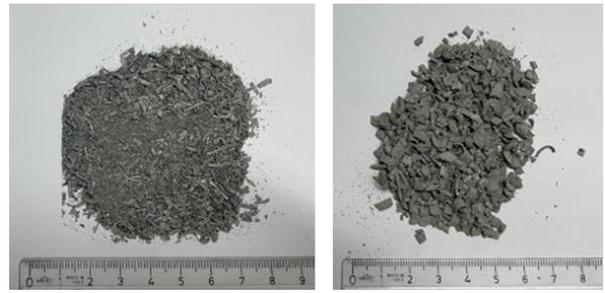
**Figure 1.** Machining waste of AlSi7Mg0.3 alloy in +2 and -2 mm size fractions.
