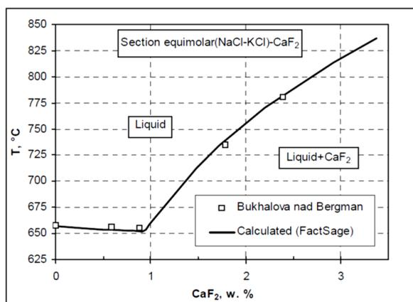
Figure 4. The ternary system NaCl.KCl-CaF<sub>2</sub> calculated by Milke et al. (2005).
