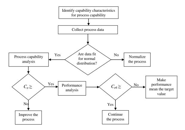
Figure 1. Flowchart of process capability analysis [15]
