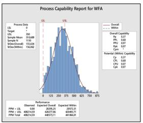
Figure 3. Process capability report for wastage fabric amount (WFA)
