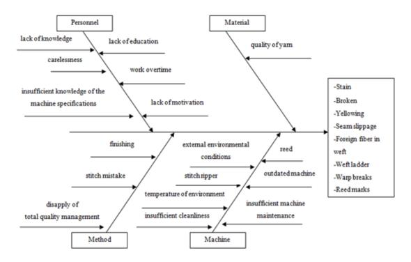
Figure 4. Cause and effect diagram for wastage fabric
