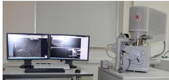
**Figure 4.** Taking SEM images of samples.
