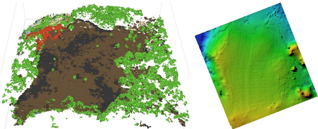
Figure 4. Classified point cloud (left) and digital elevation model (right)
