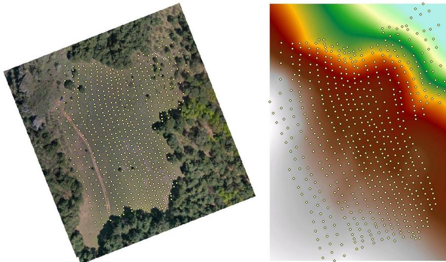
Figure 6. Total Station points (left) and Total Station based DEM (right)
