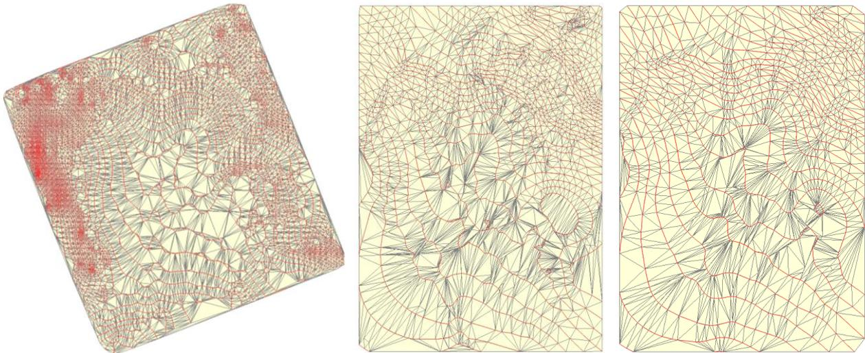
Figure 10. Triangular model and contour lines produced by UAV (left), GNSS-GPS (middle), and Total Station method (right)
