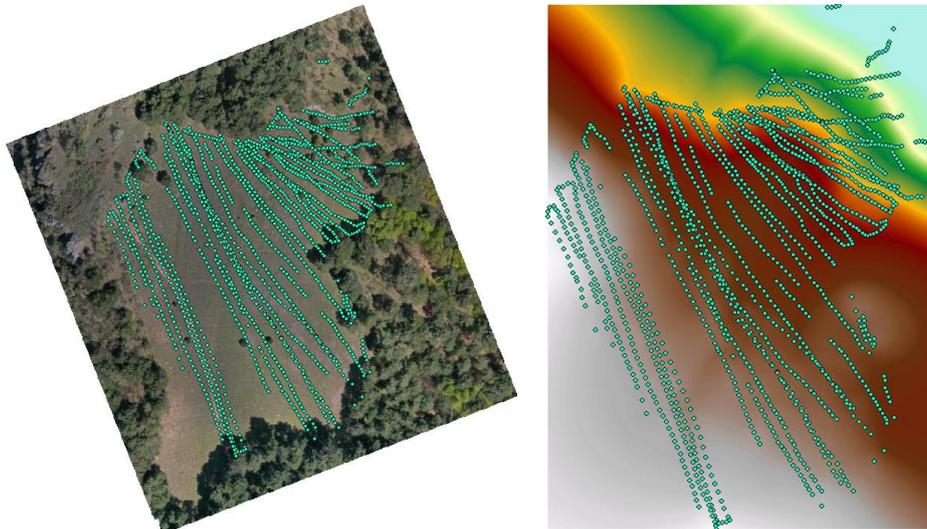
Figure 5. GNSS-GPS points (left) and GNSS-GPS based DEM (right)
