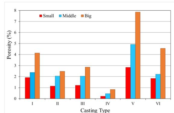
**Figure 4.** Pore values depending on casting sample section thicknesses. (I- Gravity Sand Casting, II- Casting Under Vibration, III- Sand Casting with TiB Addition, IV-Under Vibration with TiB Addition, V- Gravity Plaster Casting, VI- Casting Under Vibration)
