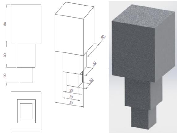
**Figure 1.** Model dimensions and solid model image.
