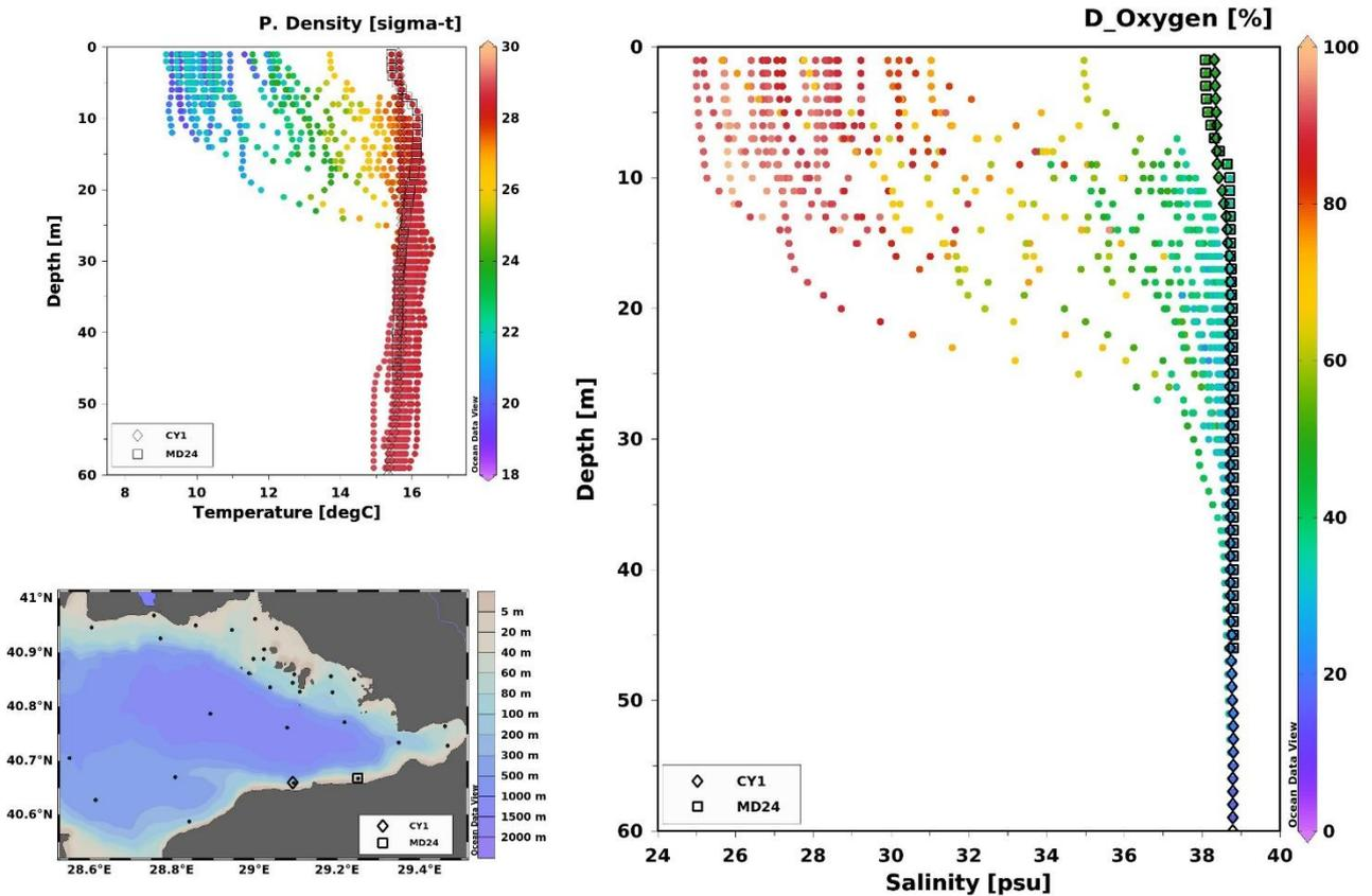
Fig. 3 The upwelling (CY1 and MD24) and neighbour stations located in the eastern part of the Sea of Marmara (left-bottom). Potential density at the surface increased even though the temperature increased at the same time (left-top). The dissolved oxygen percent decreased while the surface salinity increased because of the lower-layer rise (right).
