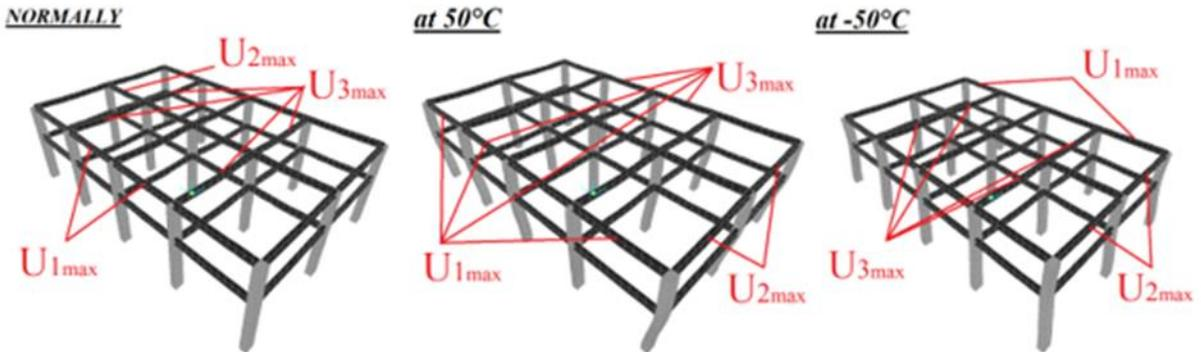
Fig. 8. Beams with maximum displacement ( $U_1$ ,  $U_2$ ,  $U_3$ ).
