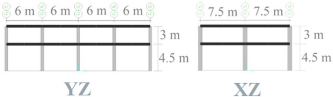
Fig. 2. The YZ, XZ plans and dimensions.
