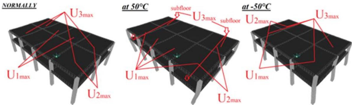
Fig. 9. Slabs with maximum displacement ( $U_1$ ,  $U_2$ ,  $U_3$ ).
