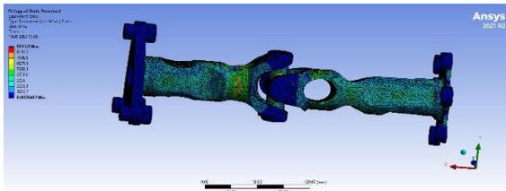
Figure 9. Stress in the optimized shaft model under boundary conditions.
