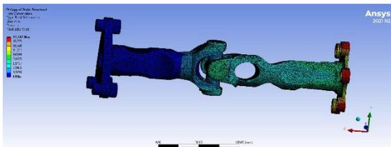
Figure 11. Deformation in the optimized shaft model under boundary conditions.
