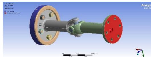
Figure 3. Boundary conditions applied to the shaft.
