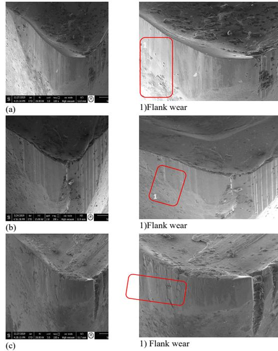
**Figure 8.**  $V = 200 \text{ m / min}$   $f = 0.2 \text{ mm / rev}$  (a) 10% soybean oil - water, (b) commercial cutting fluid, (c) wear images under dry cutting conditions
