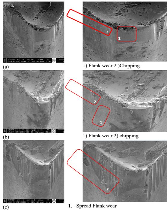
**Figure 9.**  $V = 250 \text{ m / min}$   $f = 0.2 \text{ mm / rev}$  (a) 10% soybean oil - water, (b) commercial cutting fluid, (c) wear images under dry cutting conditions
