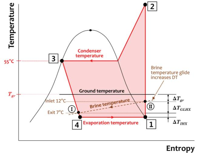
Figure 7. a) Working principle of a GSHP system for both heating and cooling mode b) T-S diagram [192].
