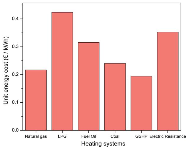
**Figure 1.** Energy consumption costs for the different heating system [18].
