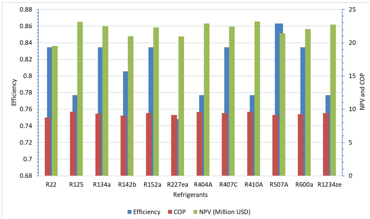
**Figure 9.** Maximum performance of 12 different working fluids [195].
