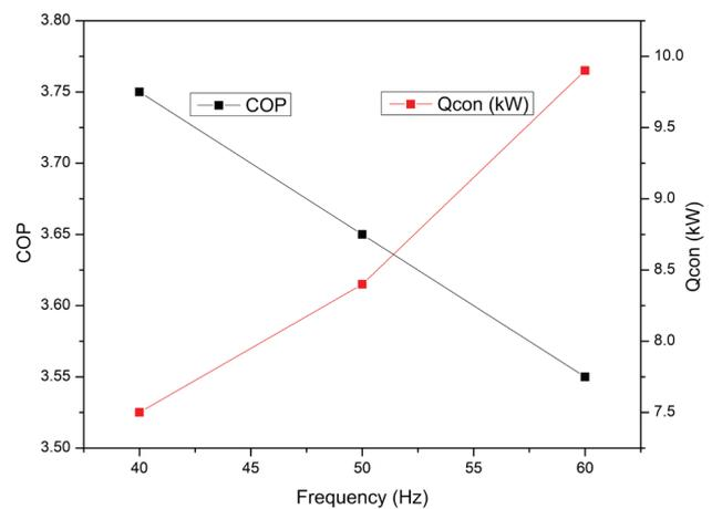
Figure 8. The effect of supply voltage frequency on performance and condenser load at an evaporator temperature of  $-2.5\text{ }^{\circ}\text{C}$  [104].
