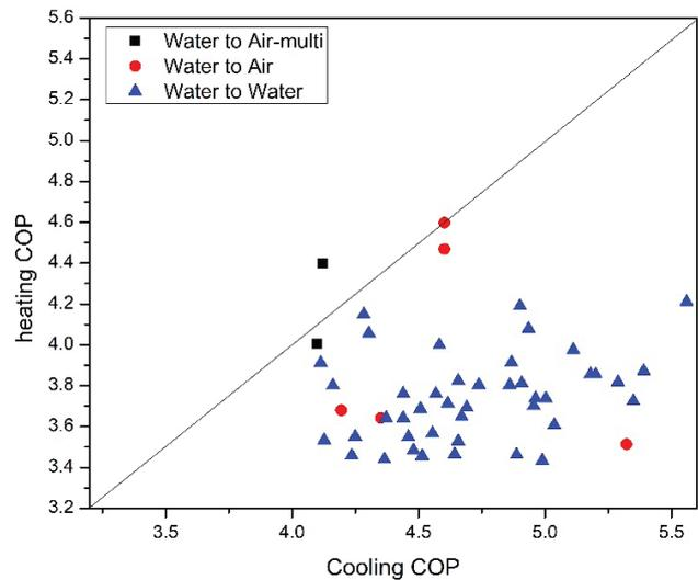
**Figure 10.** Variation of heating and cooling COP for a different type of heat pump [218].
