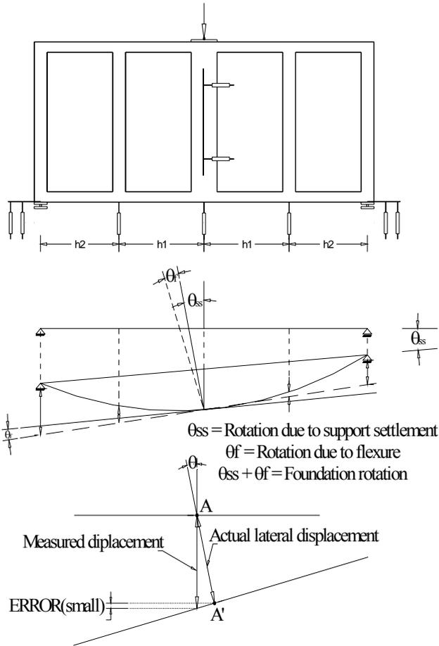
Figure 4. Calculation of the lateral deflections (twin frames)
