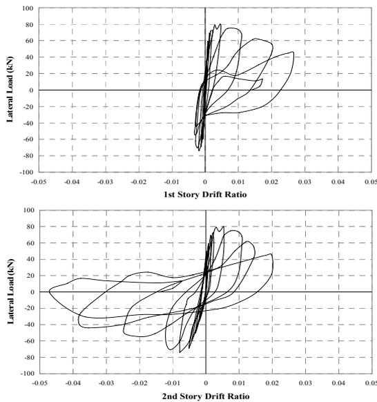
Figure 9. Drift ratio-lateral load graphs for both stories (Specimen PPR1)
