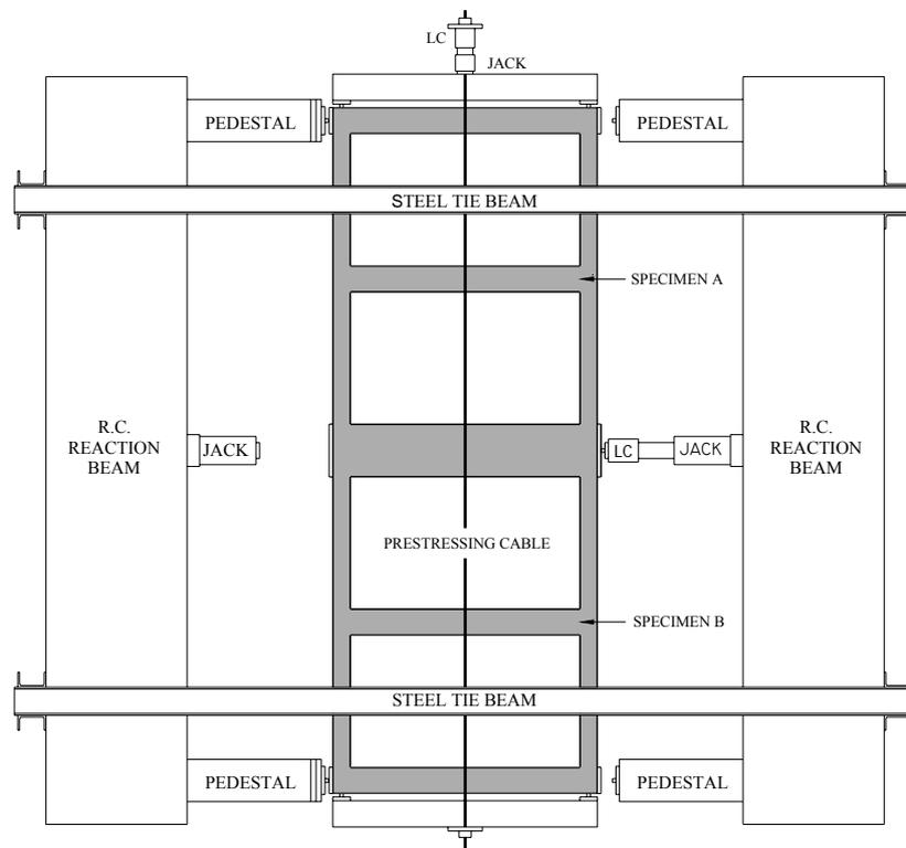
Figure 1. Test set-up of twin frames
