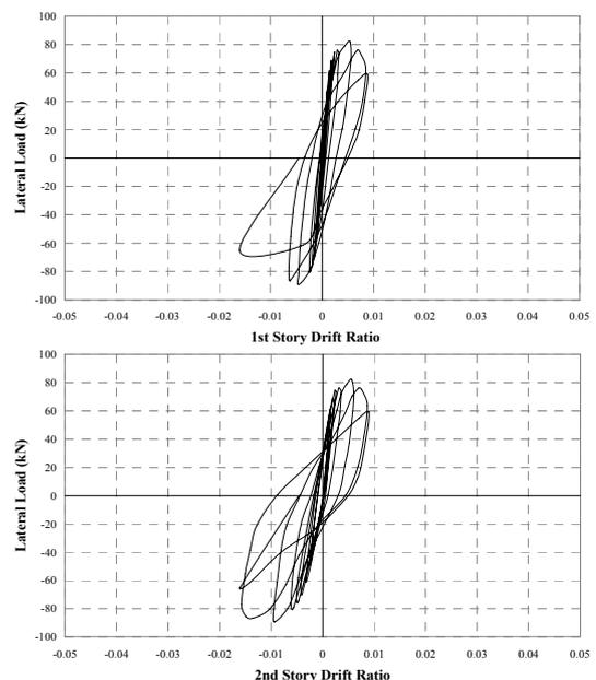
Figure 12. Drift ratio-lateral load graphs for both stories (Specimen PPR2)
