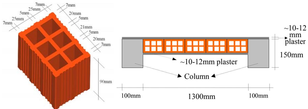
Figure 7. Hollow Brick Used as Infill Material and Infilling Method
