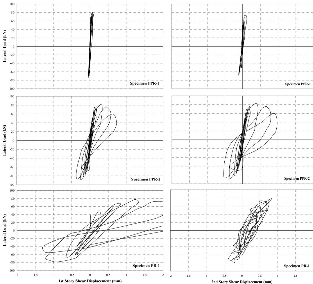
Figure 18. Infill wall shear displacements – Lateral load graphs of the test specimens
