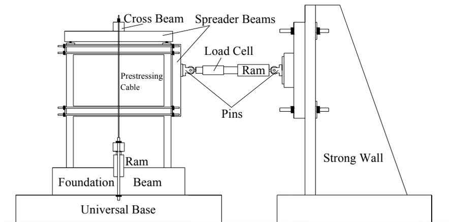
Figure 15. General view of the newly developed test set-up (last form)
