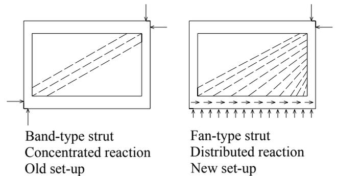
Figure 11. Reaction types developing at the foundation level
