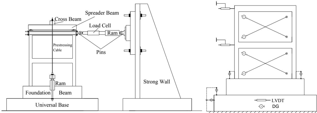
Figure 8. General view of the newly developed test set-up and instrumentation
