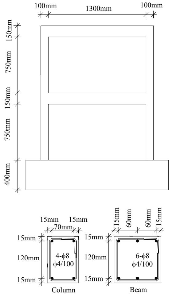
Figure 6. Dimensions and reinforcement of the test frames
