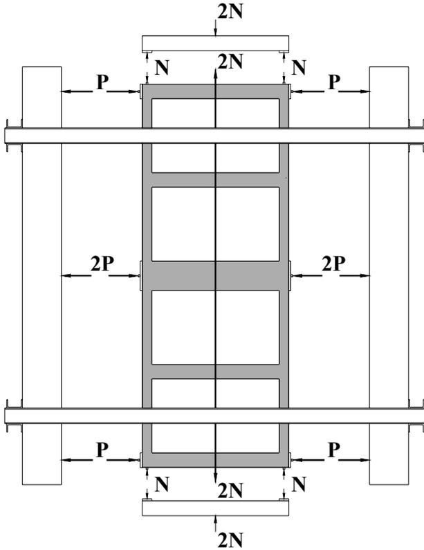
Figure 2. Forces acting on the twin frames
