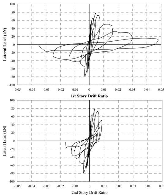
Figure 16. Drift ratio-lateral load graphs for both stories (Specimen PR1)
