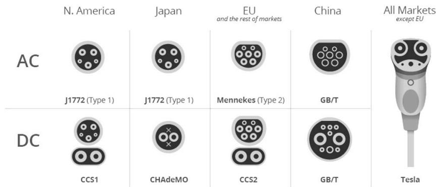
**Figure 2.** Connector types [22].
