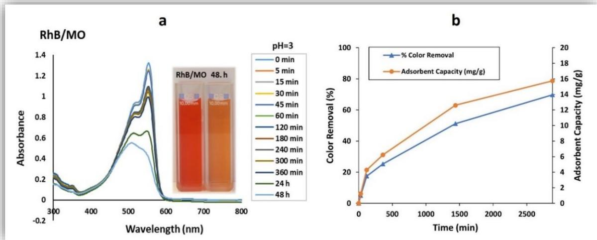
**Figure 5.** a) Time-dependent UV-Vis absorption spectra of the aqueous solution of RhB/MO treated by **Hg-CP** at pH=3. b) Time-dependence of adsorption profiles of RhB/MO over **Hg-CP** at pH 3.
