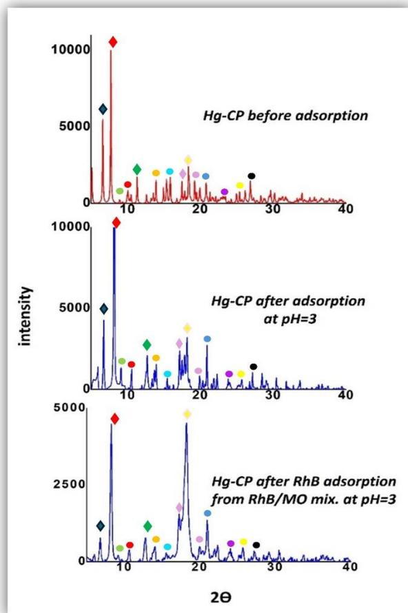
**Figure 7.** Matched-PXRD diffractogram of **Hg-CP** before and after adsorption.
