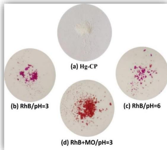
**Figure 6.** For **Hg-CP** (a) before adsorption, (b) after RhB adsorption at pH=3, (c) after RhB adsorption at pH=6, (d) after RhB+MO adsorption at pH=6.
