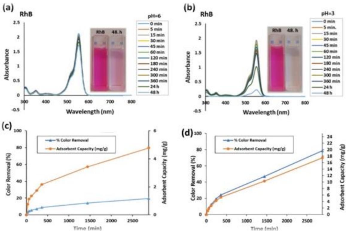
**Figure 2.** Time-dependent UV-Vis spectra of the aqueous solution of RhB treated by at pH=6 (a), pH=3 (b) and time-dependence of adsorption profiles of RhB over at pH 6 (c) and pH=3 (d).
