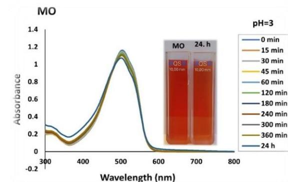
**Figure 4.** UV-Vis absorption spectra of the aqueous solution of MO treated by **Hg-CP** with time dependence at pH=3.
