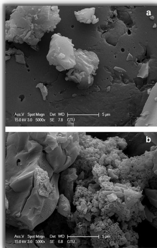
**Figure 8.** SEM image of **Hg-CP** before (a) and after (b) adsorption.
