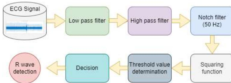
Figure 5. Pan-Tompkins algorithm block diagram.
