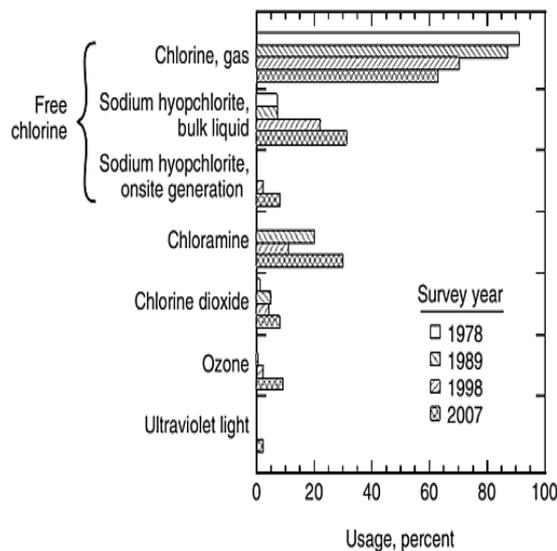
Figure 1. The chemicals used for disinfection [1]
