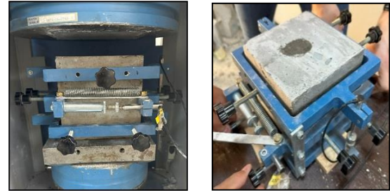
Figure 6. Determination of stress-strain relationship of mortar material
