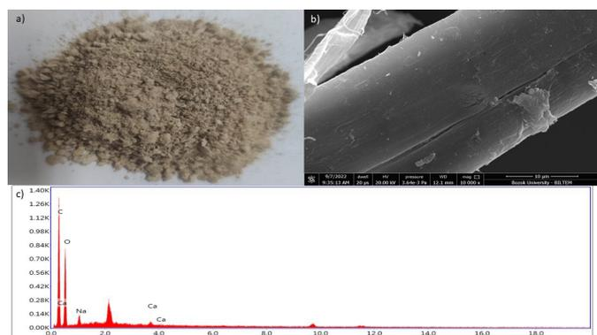
**Figure 2. a)** Image of Processed Fiber, **b)** SEM Image of Processed Fiber, **c)** EDX Analysis of Processed Fiber
