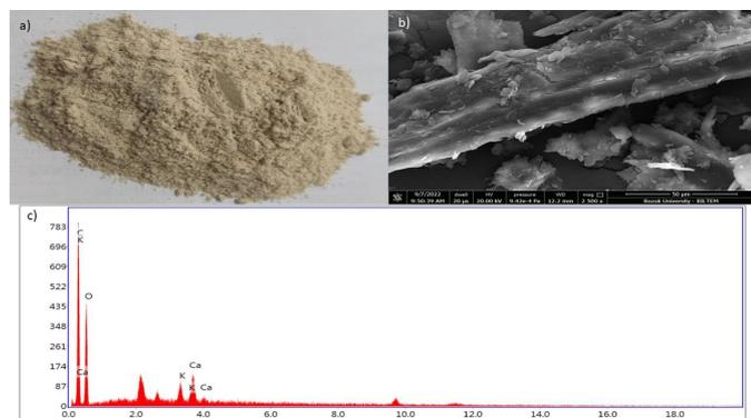
**Figure 1. a)** Image of Ground Raw Fiber, **b)** SEM Image of Unprocessed Raw Fiber, **c)** EDX Analysis of Unprocessed Raw Fiber
