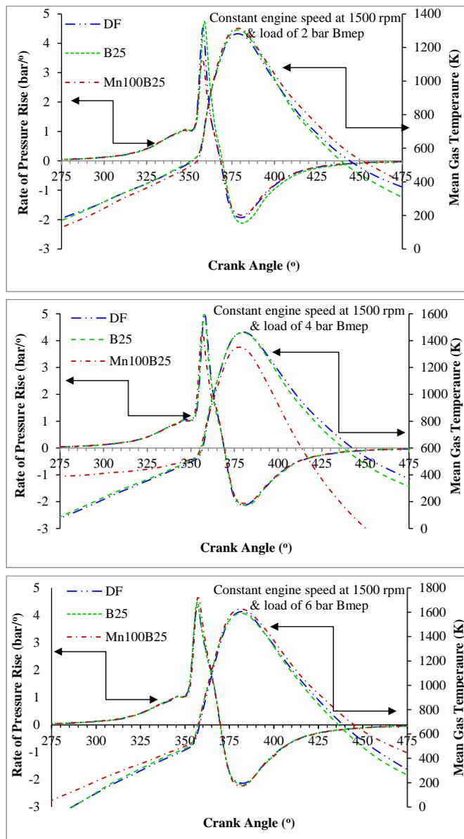
Figure 3. The mean gas temperature curves and rate of pressure rise curves under varying loads
