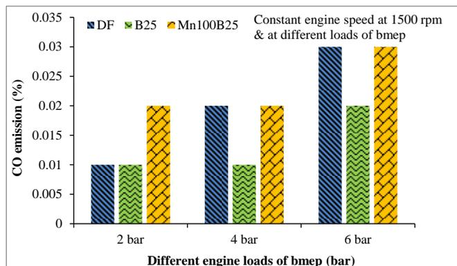
Figure 6. The variation of CO emissions under varying loads for test fuels
