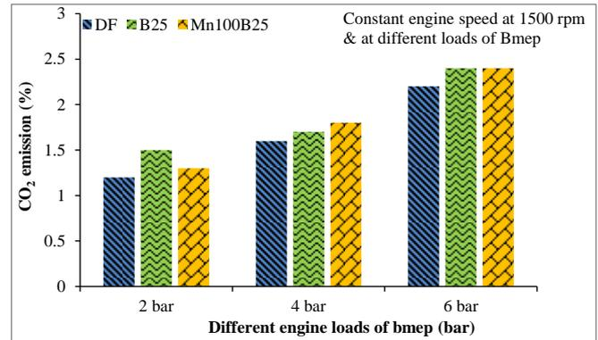
Figure 7. The variation of CO<sub>2</sub> emissions under varying loads for test fuels
