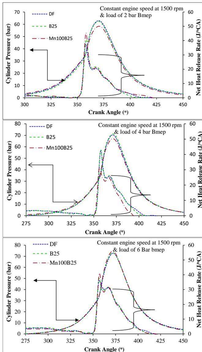
**Figure 2.** Cylinder gas pressure and net heat release rate curves under varying loads
