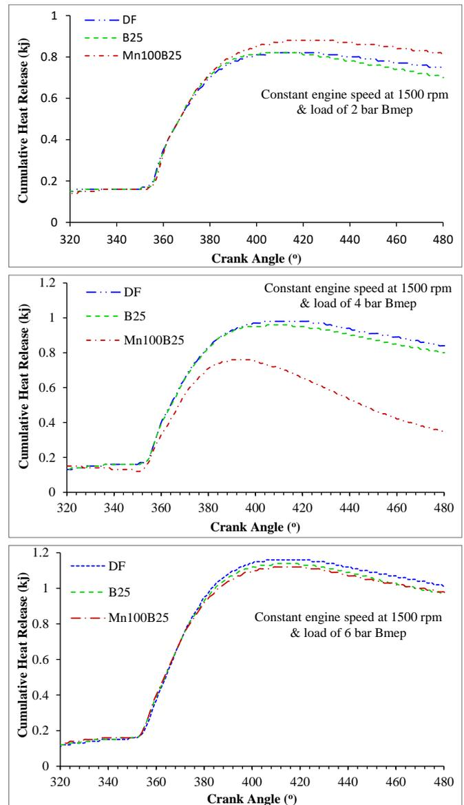
Figure 4. The cumulative heat release curves under varying loads
