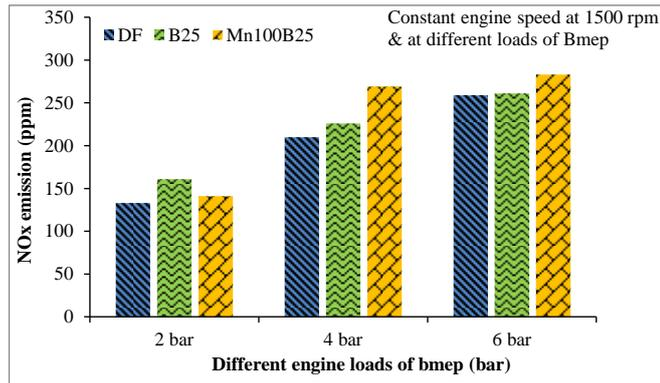
Figure 5. The variation of NO<sub>x</sub> emissions under varying loads for test fuels
