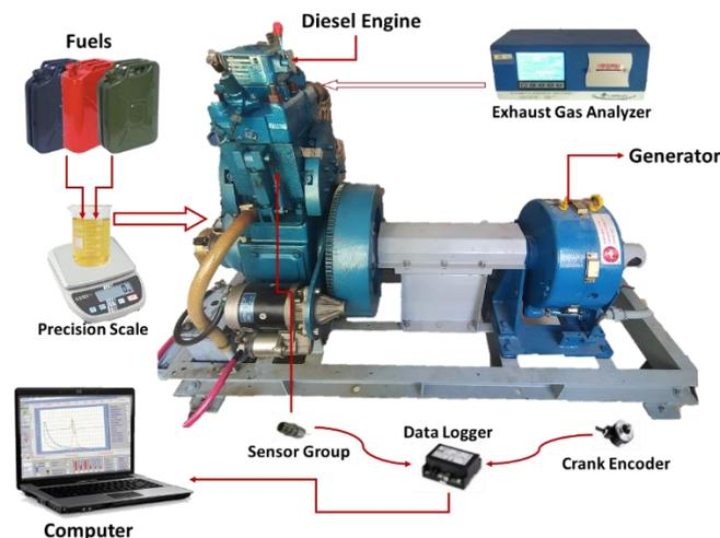
Figure 1. Schematic view of the experimental engine
