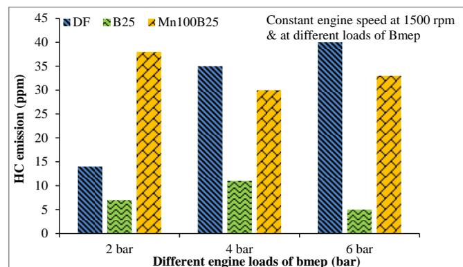
Figure 8. The variation of HC emissions under varying loads for test fuels
