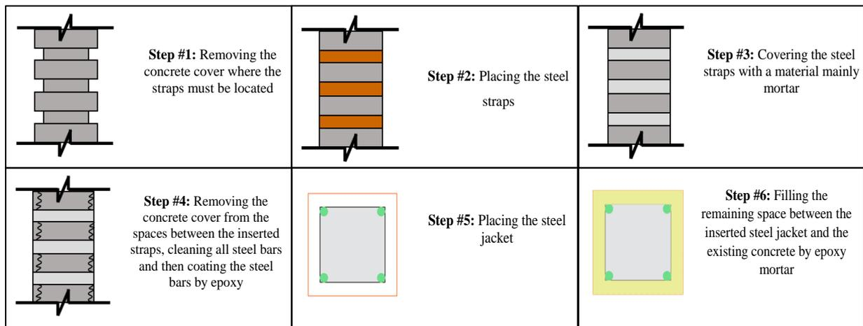
**Figure 2.** Steel jacking of concrete columns procedure [41]
