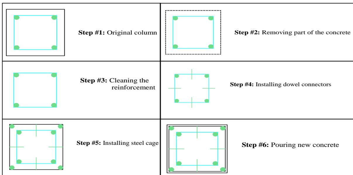
**Figure 6.** Steps of concrete jacketing process [58]
