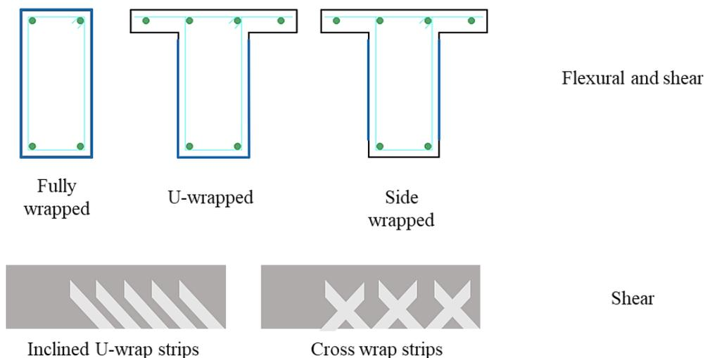
**Figure 9.** Fiber reinforced polymer techniques [104]
