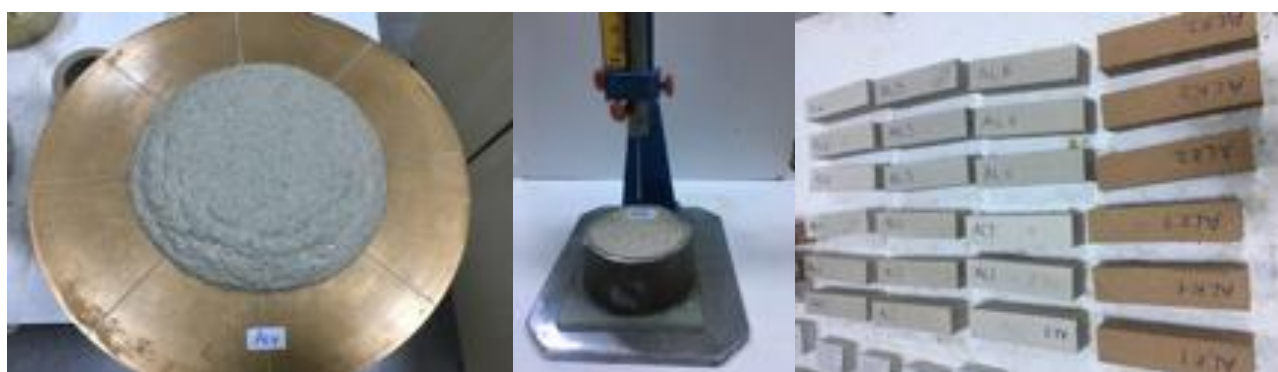
Figure 1. The views from flow table, setting time and hardened mortar samples.
