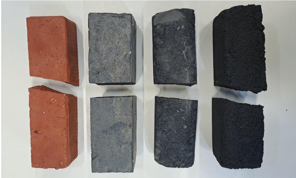
Figure 1. Broken sample bricks after three-point flexural test
