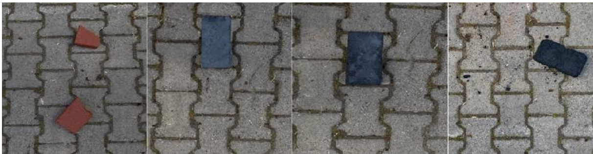
Figure 3. a) Impact test result of red brick b) Impact test result of S1 c) Impact test result of S2 d) Impact test result of S3
