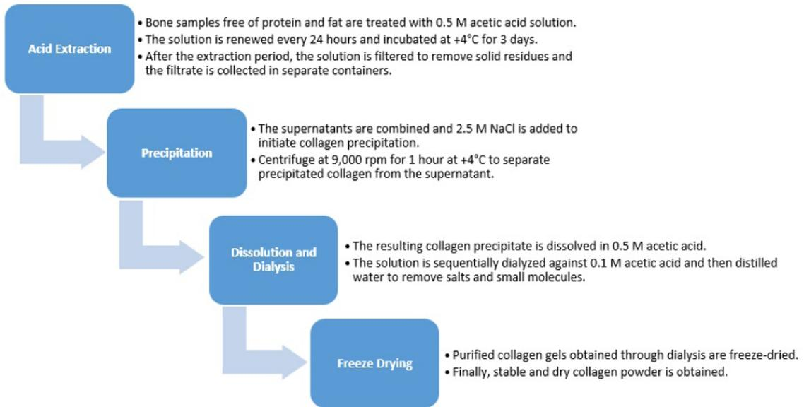
**Figure 3.** Extraction procedure for collagen isolation from fish bones.
