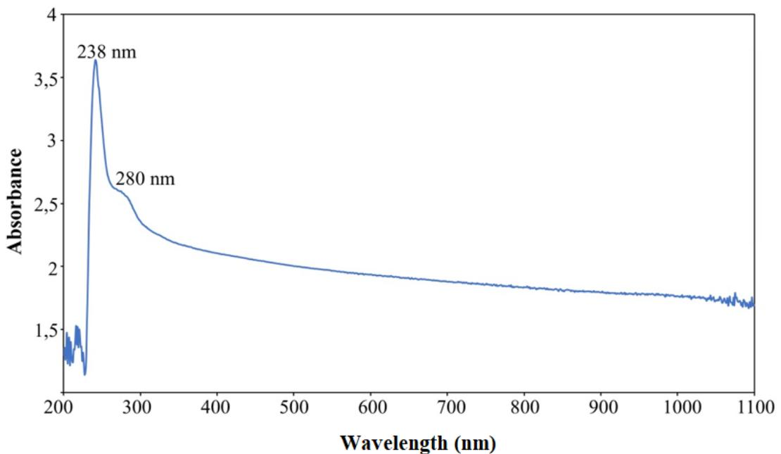
**Figure 4.** The UV absorption spectrum of collagen from fish wastes.
