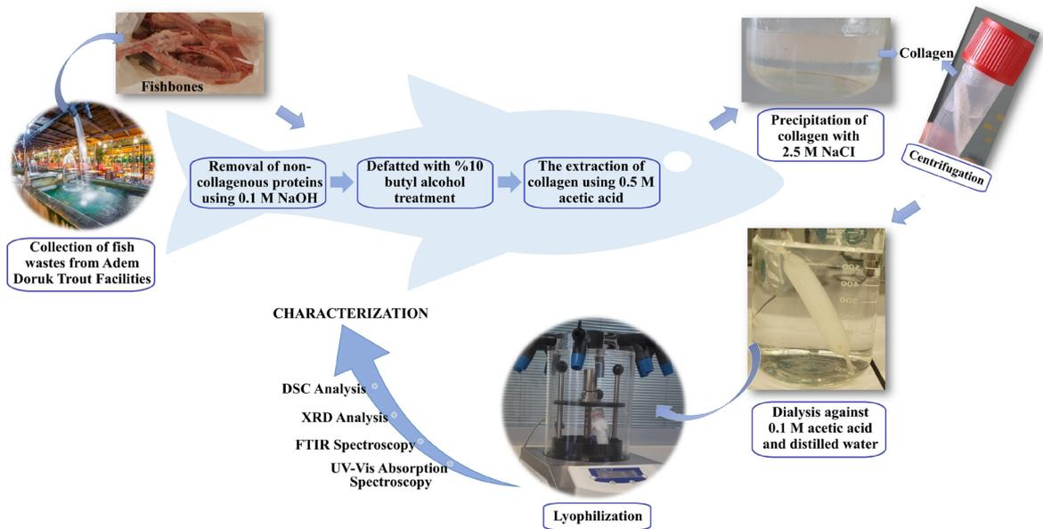
**Figure 1.** Schematic representation of the processes of collagen extraction.
