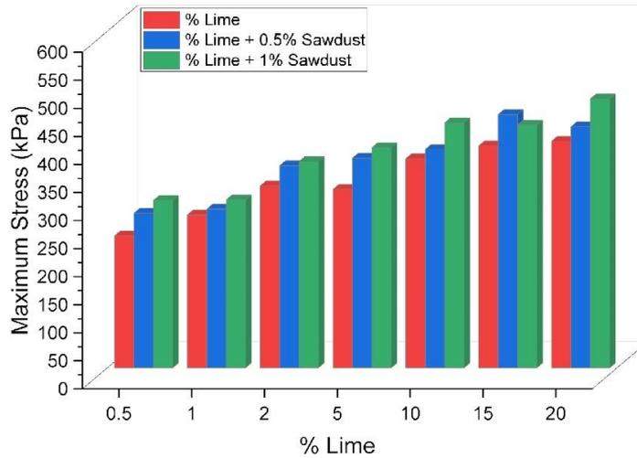
**Figure 4.** Unconfined compression test results with 30 % water content concerning Sample-2
