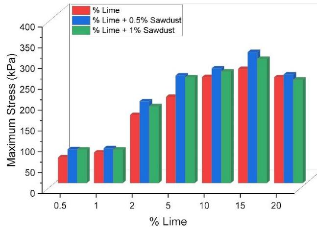
**Figure 2.** Unconfined compression test results with 30 % water content concerning Sample-1
