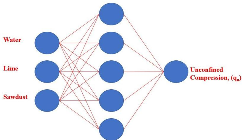
**Figure 5.** Architecture of the Neural Network model for prediction
