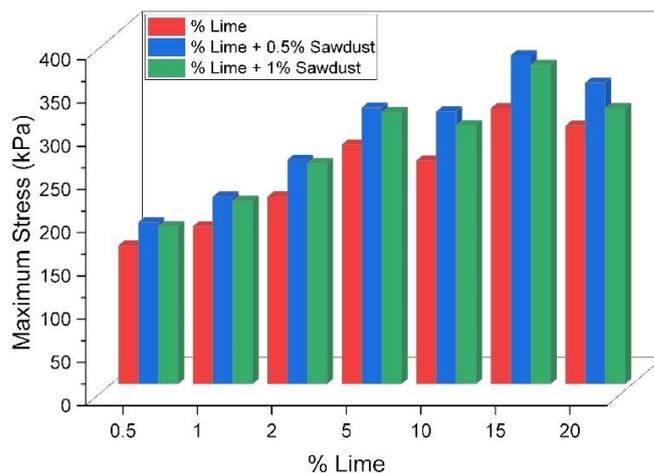
**Figure 1.** Unconfined compression test results with 25% water content concerning Sample-1
