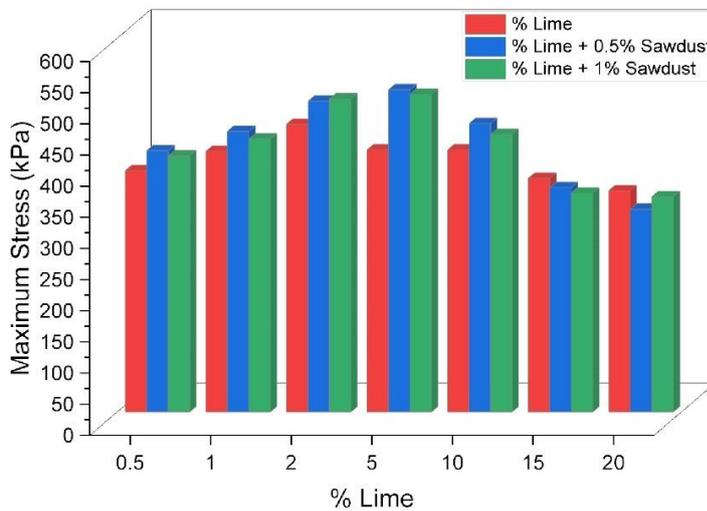
**Figure 3.** Unconfined compression test results with 25 % water content concerning Sample-2
