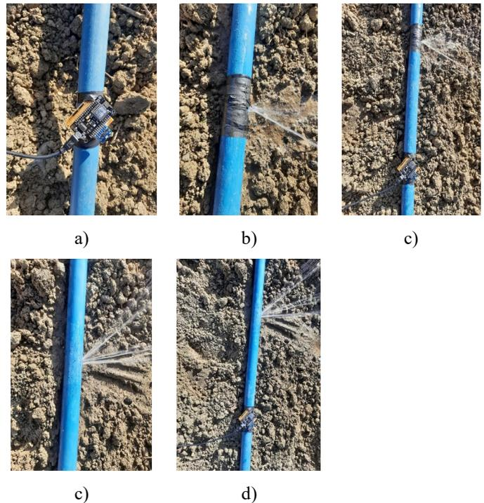
**Figure 8** Collecting data on solid and perforated pipes a) Placing the sensor module on the solid pipe b) Perforated pipe c) Placing the sensor module on the perforated pipe d) Multi-hole pipe e) Placing the sensor module on the multi-hole pipe
