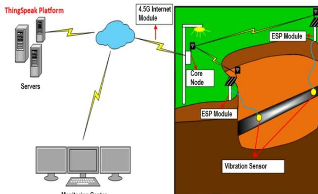
**Figure 5** IoT-based data collection platform developed within the scope of the study
