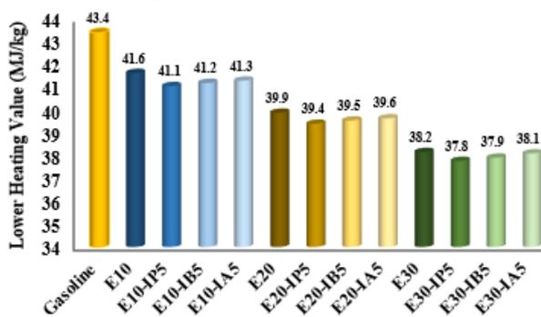
Figure 4: Lower heating value of fuel samples.
