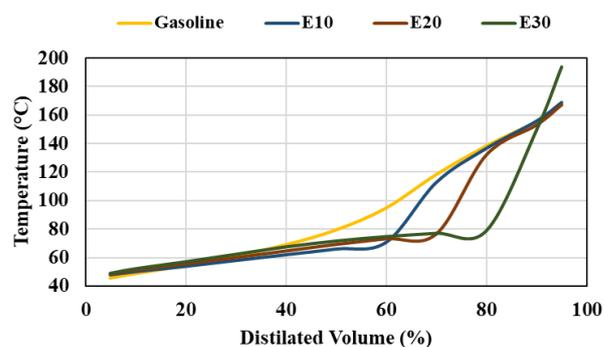
Figure 6: Distillation curve of gasoline and ethanol-gasoline mixtures.
