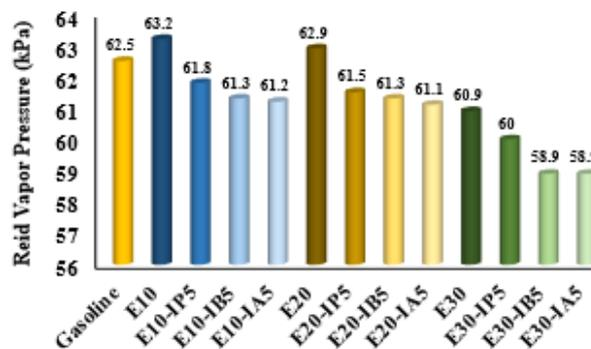
Figure 2. Effect of adding C3-C5 iso-alcohols on the vapor pressure of the ethanol-gasoline mixtures.
