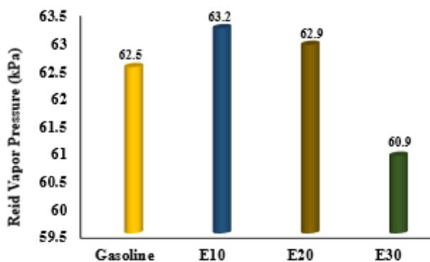
Figure 1. RVP of gasoline and ethanol-gasoline blends.
