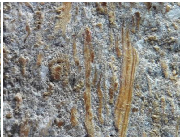
Figure 8. Wood-cement compatibility effect.
