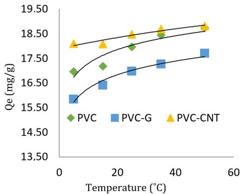
**Figure 7.** Effect of temperature (Initial dye conc.: 250 mg/L, pH: 5.0, ads. dose: 3,00 g/L).
