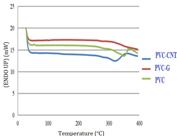
Figure 5. DSC graphs of pure, carbon nanotube-doped, and graphene-doped PVC nanofiber membranes.
