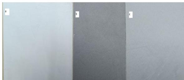
**Figure 2.** Nanofiber membranes obtained from PVC polymer, a) Pure PVC Nanofiber membranes, b) 2% carbon nanotube-doped PVC nanofiber sheets, c) 2% graphene-doped PVC nanofiber sheets.
