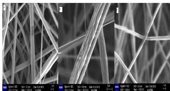
**Figure 3.** SEM Analysis a) PVC b) PVC-CNT c) PVC-G nanofibers.
