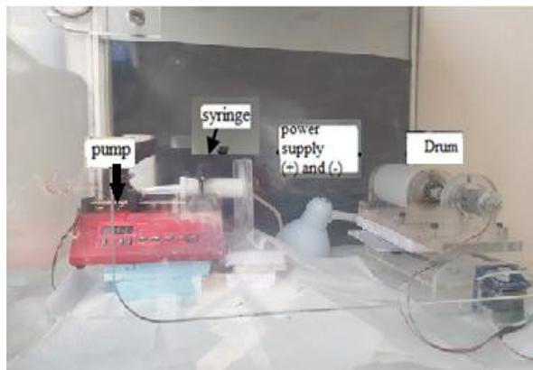
**Figure 1.** Electrospinning device used in nanofiber production.
