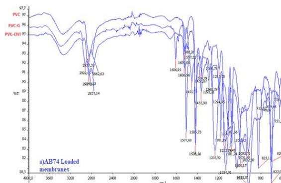
**Figure 4.** a) IR spectra for AB74 loaded nanofiber membranes.
