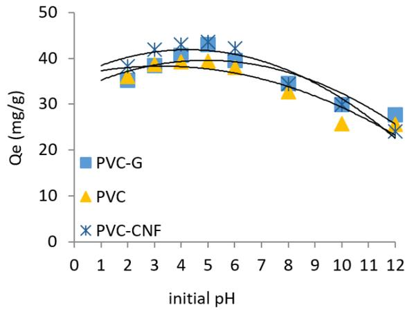
**Figure 6.** Effect of initial solution pH on adsorption of AB74 (Initial dye concentration: 250 mg/L, ads. dose: 3.0 g/L, agitation time: 10 h).
