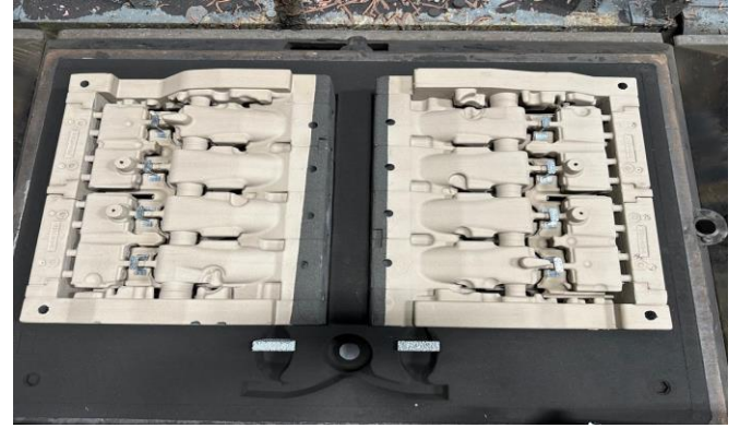
Figure 1. Core and filter placement before molding of engine blocks.
