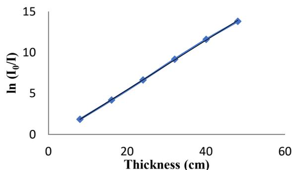
Figure 1. Plot of  $\ln(I_0/I)$  versus attenuator material thickness (for Sample 3, %50 PbO, and 1332 keV gamma rays)
