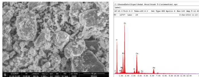
**Figure 7.** The results of Sem-EDS Analysis of clay type
