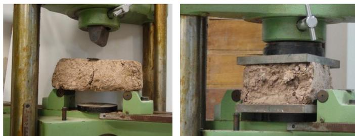
**Figure 8.** The mechanical property test photos of Adobe samples
