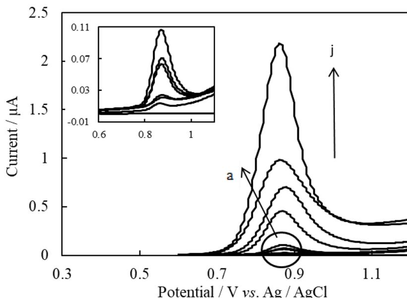
**Figure 6:** SWAAdS voltammograms of NZ HCl at different concentrations (in  $\mu\text{mol L}^{-1}$ ) a: 0.05, b: 0.08, c: 0.1, d: 0.5, e: 0.8, f: 1.0, g: 5.0, h: 8.0, i: 10.0, j: 30. Inset: SWAAdS voltammograms from a to f.
