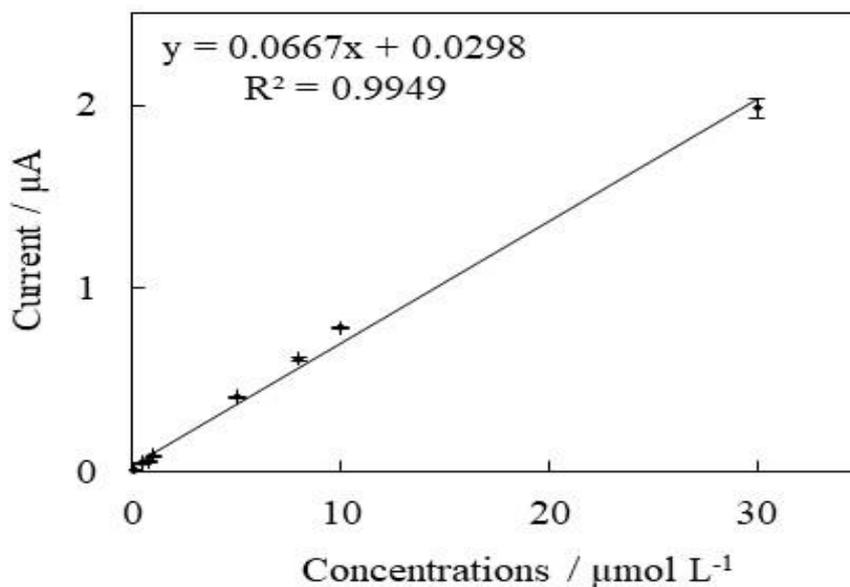
**Figure 7:** Calibration curve for NZ HCl solutions in BR buffer of pH 7.0 ( $t_{\text{deposition}}$ : 90.0 s,  $E_{\text{deposition}}$ : 0.6 V). Error bars show the standard deviation of three measurements.
