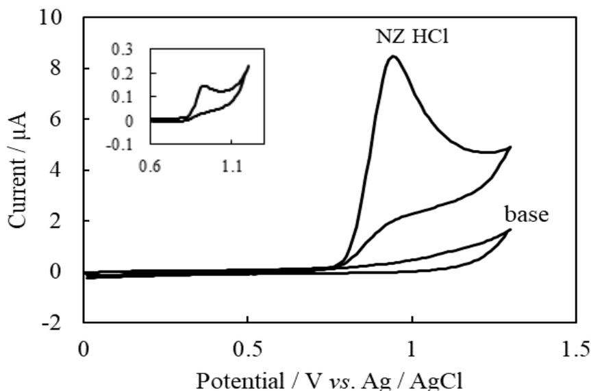
**Figure 2:** Cyclic voltammograms of  $1.5 \times 10^{-3}$  mol L<sup>-1</sup> NZ HCl solutions at Al<sub>2</sub>O<sub>3</sub>-NPs-CPE in BR buffer solution pH 7.0 and scan rate 0.1 V s<sup>-1</sup> (inset: cyclic voltammograms of NZ at bare CPE at the same condition).
