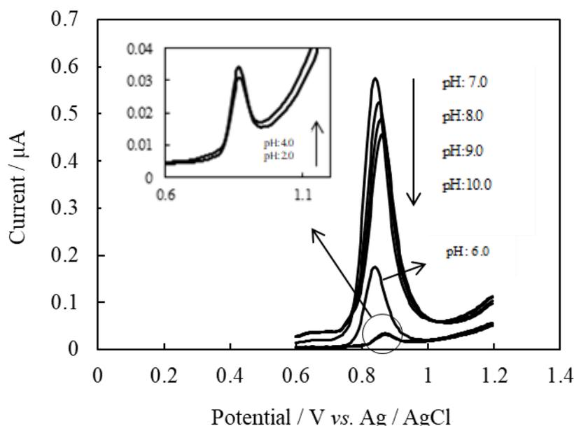
**Figure 5:** Effect of pH on SWVs of  $1.0 \times 10^{-5}$  mol L<sup>-1</sup> NZ HCl. Inset: SWVs obtained at pH 2 to 4.
