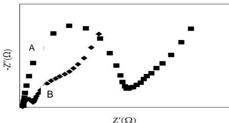
**Figure 4:** The Nyquist curves of (A) UCPE and (B) Al<sub>2</sub>O<sub>3</sub>-NP-CPE in 0.1 M KCl solution containing 5.0 mM Fe(CN)<sub>6</sub><sup>3-/4-</sup>.
